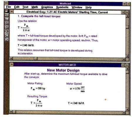
The Electronic Handbook in the top window is opened to the calculations for determining the fully loaded torque of an AC motor. The bottom window shows a working document where the user is calculating some of the properties for a new conveyor design. To copy the formula from the Handbook to the working document just requires double-clicking on the Handbook formulas.
