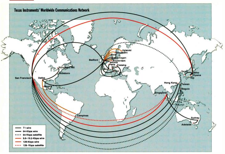
**Texas instruments' global** communications network illustrates just how complex worldwide networking can get. The LAN internetwork spans several different transmission methods, from dedicated modem lines to satellite links.
