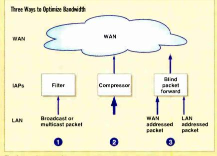
**The three main approaches** to squeezing the most out of expensive WAN bandwidth are: • Filter broadcast and multicast overhead traffic from entering the WAN. • Compress the size of packets before they are transported over the WAN. • Pass only those packets that do not possess a local network layer address (blind packet forwarding).
