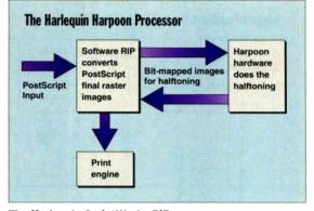
**The Harlequin ScriptWorks RIP** works hand in hand with the Harpoon processor to increase the throughput and enhance the image of PostScript files. The Harpoon processor deals only with the halftoning process.
