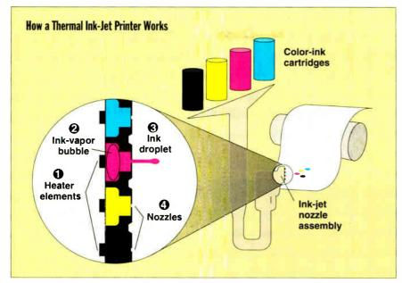
**Thermal ink-jet printers** use heat  $\bullet$  to create a vapor bubble @ that forces a droplet of ink  $\bullet$  through a nozzle  $\bullet$ .
