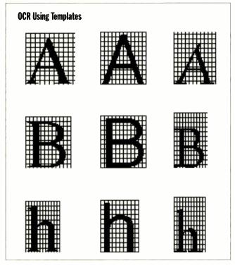
Several typefaces broken up into 10- by 10-pixel grids for recognition.
