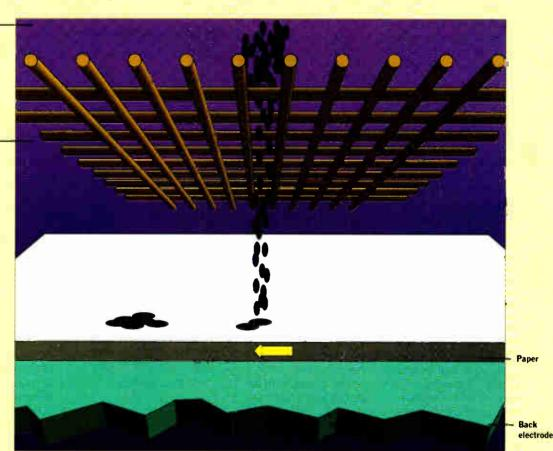
**Array's Tonerlet by Array technology** places an electrically charged control electrode array, which can be either a wire mesh or a perforated flexible printed circuit board, between the toner and the paper. A back electrode beneath the paper attracts toner and pulls it through the holes in the control electrode array. The toner lands on the paper and forms a dot.
