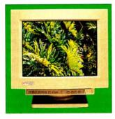
monitor has a horizontal frequency scan rate of 30 to 65 kHz that supports noninterlaced resolutions of up to 1280 by 1024 pixels; its 1024- by 768-pixel resolution has a 76-Hz refresh rate. The 2000DC is VESA DPMS compliant and meets Energy Star guidelines.
