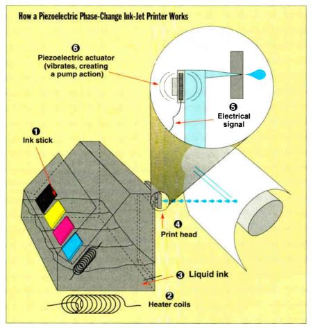
**Piezoelectric phase-change ink-jet printers** use a solid ink **O**. A heating element **O** melts that ink **O**, which then goes to the actuator in the print head **O**. Pulses of electricity **O** create a pumping action in the actuator **O**, and this forces the ink out onto the paper. The ink then solidifies as soon as it touches the paper, avoiding the spreading, or wicking, problems associated with liquid inks.
