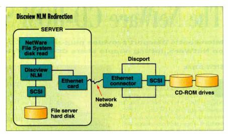
**The Discport attaches** as a network node, but CD-ROM drives attached to it appear logically attached to a server due to Microtest's NLM. The NLM on the server reroutes CD-ROM accesses directed at the server to the Discport, which translates between Ethernet packets and SCSI-2 blocks.
