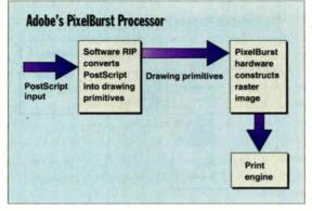
**The Adobe PixelBurst processor** can significantly boost the processing speed of raster files. It uses the list of drawing primitives produced by the software RIP to construct the raster image sent to the printer.
