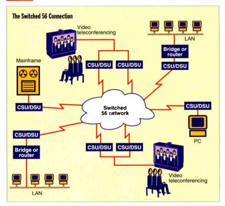
**Switched 56 connections** can serve most applications that demand high-speed communications: videoconferencing, network interconnectivity, or mainframe links. Each end of the connection must have a CSU/DSU and perhaps a bridge or router.
