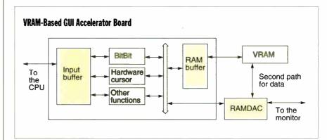
The second port on the VRAM allows the data to flow to the display device at the same time that new drawing information arrives from the GUI acceleration hardware.
