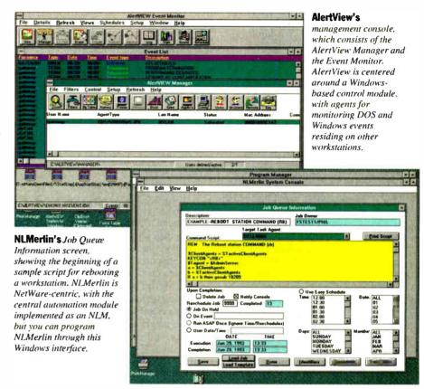
itor events, schedule and initiate procedures, and gain control of workstations through the workstation agents. The agents monitor system events and report them to the management console. All modules communicate via IPX, DLC (data-link control), NetBIOS, or TCP/IP and proprietary packets.
