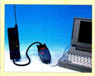
The I.D.E.A. (Intelligent Data Equipment Adapter) lets you connect your modem or fax machine to a portable cellular phone. Powered by a standard 9-V battery, the I.D.E.A. (from \$249.95) gives your cellular phone the characteristics of a standard phone line. The microprocessor-controlled system generates a dial tone, controls the functions of the phone, and provides a standard RJ-11 interface. The system, which is compatible with PCs, Macs, and palmtops, does not require additional software.
