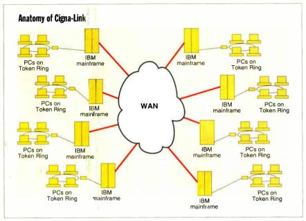
A simplistic view of Cigna-Link, Cigna's WAN (wide-area network) infrastructure. Each office runs PCs over a Token Ring network. The Token Rings talk to an IBM mainframe. The mainframes are connected with an IBM SNA network over T1- and T3-grade leased phone lines.
