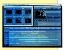
based interface and then record the finished program back onto videotape. Media 100's video output is 60 fields and 30 frames per second. The system, which consists of two NuBus boards and video-production software, supports input and output of four independent tracks of CD-quality stereo audio.
