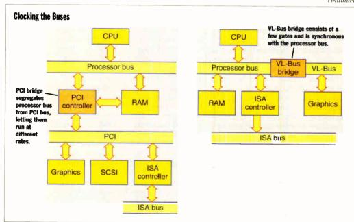
crosoft's Video for Win- VL-Bus requires a simple bridge to the processor bus, allowing it to run synchronously with the processor. PCI has a dows, which incorporates complicated bridge and runs asynchronously,
