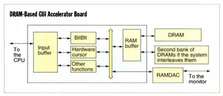
The screen image must flow back through the accelerator hardware before it is sent to memory, causing conflicts with screen-drawing information.
