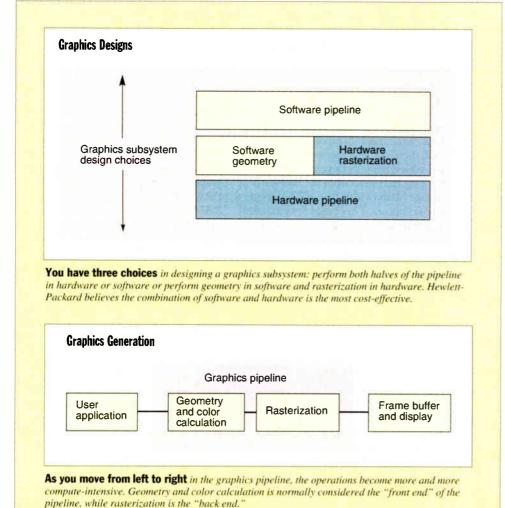
the most expensive option—typically out of the price range of average users. In fact, it is not uncommon for a graphics subsystem using this approach to cost more than the CPU it connects to. Moreover, performance is forever stuck at the level that the dedicated hardware pipeline provides, and it doesn't scale up with advancing CPU performance.
