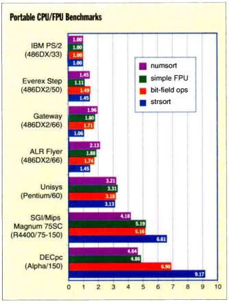
**BYTE's portable benchmarks** display raw CPU/FPU horsepower for five Intel systems and two RISC machines.
