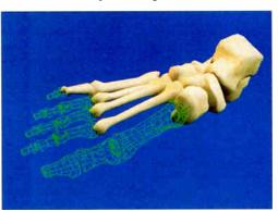
An important feature of the Sun SparcStation ZX graphics architecture used to render the photo is its ability to perform dynamic tessellation of NURBS (nonuniform rational B-splines) curves and surfaces. NURBS are concise, yet powerful, representations of simple and complex geometries. From a high-level mathematical description, the graphics system tessellates curved geometry into lines (in the case of curves) or triangles (in the case of surfaces).
