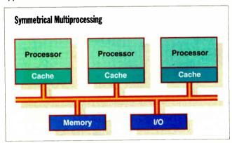
In a symmetrical multiprocessing system, the processors have equal access to system resources, and any processor can run any operatingsystem or application thread. In an asymmetrical system, one processor usually runs the operating system and controls access to resources, creating imbalances in the distribution of work across the processors in the system.
