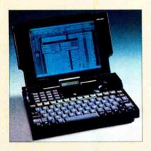
When BYTE last looked at the Olivetti Quaderno (see "Ultraportable PCs: Worth the Trade-Offs?," April BYTE), we found that it filled a niche somewhere between a bulky palmtop and an underpowered subnotebook. With an 8086-compatible V30 chip running at 16 MHz, 1 MB of RAM, a 20-MB hard drive, and a reflective LCD screen, the Quaderno could run DOS, but you couldn't touch-type on the diminutive keyboard.
