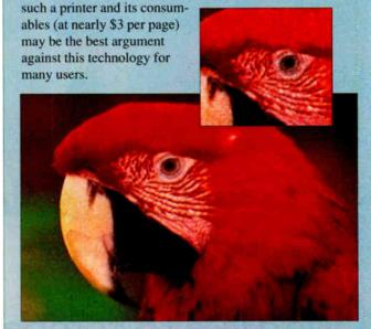
The image on the bottom was produced by the Tektronix Phaser IISDX, the dye-sublimation model with the highest quality score of any color printer we tested. On the top is output from the Tektronix Phaser 2001, a high-quality thermal-wax-transfer printer. Note: Both images were magnified 150 percent to illustrate the dot structure of thermal-wax-transfer printers versus the continuous tones of dye-sublimation technology.
