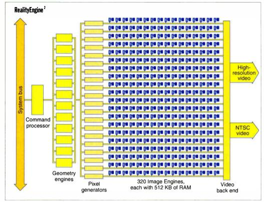
With the processing bandwidth of a supercomputer, the RealityEngine<sup>2</sup> uses parallelism to achieve real-time texture mapping and antialiasing of 3-D images.
