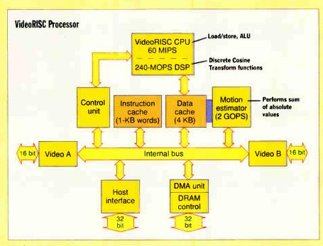
**The functional units** of the VideoRISC processor are designed to perform the types of computations required by compression and decompression algorithms.
