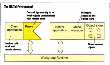
The DSOM Environment lets applications take advantage of remote objects by creating a local proxy that regulates access to remote methods.
