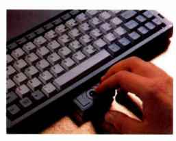
The integrated track ball slides out from a compartment by the space bar on the keyboard. You simply pull it out and go to work. Finished? Just slide the track ball back into the ColorBook.
