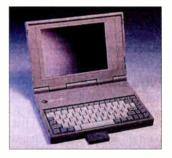
an 80- or 170-MB hard drive, an integrated trackball, and a PCM-CIA Type III slot.
