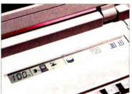
er or in time remaining) and what level of power management you've set. Other icons show typical items such as Caps-Lock, floppy drive and hard drive access, and whether the power is on
