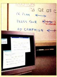
in real time the position of the markers you use to write on the board. They then translate the data onto your computer display. You can set up multisite sessions using a modem and standard phone lines.
