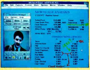
A Cadillac among desktop video and document conferencing systems, NCR's TeleMedia Connection is a hardware and software package that supports collaborative document mark-up and real-time video-in-a-window, It uses H.261-standard compression and requires dual ISDN channels for quarter-screen video throughput of 15 fps.
