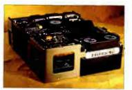
that fits more controller electronics onto the board by wrapping the flexible printed circuit board around the drive mechanics. (This same technology is often found in notebook computers.)
