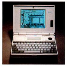
The Subnote is a high-powered machine manufactured for CompUSA by Taiwan-based Twinhead. Of the three reviewed systems, the Subnote is the only one built around a 486-class processor, and the only one with an FPU. Although not as radical in innovation as the others, the Subnote is a solid performer, easily portable, and in-expensive—a 4-MB RAM, 80-MB hard drive model costs just \$1999.
