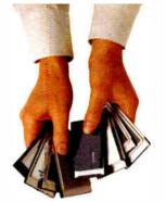
Two PCMCIA 2.01 Slots, Type II (5mm) and 16mm: Twice the expandability. Easily accepts multiple cards including hard disk drives, modems and networking adapters.
