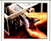
You install the 1.2 meg, 5-1/4" floppy disk drive, learning disk drive operation and adjustment. Later, you dramatically improve your compu-ter's data storage capacity by instal-ling a powerful 80 meg IDE hard drive.
