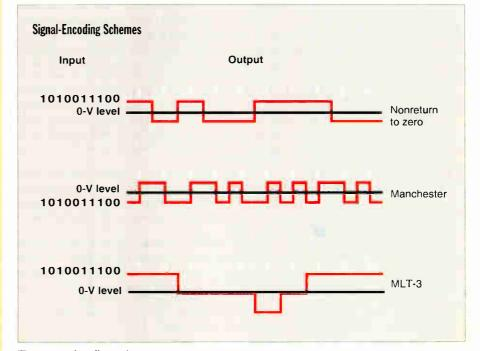
The way a signaling scheme represents strings of bits determines the electrical characteristics of a network. Although complex signaling schemes (e.g., MLT-3) have greater processing overhead. they can reduce electrical noise by decreasing the voltage changes necessary to transmit a signal.
