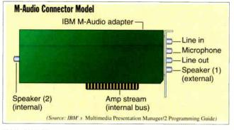
**IBM's MMPM/2** uses connectors to indicate the way in which data is transferred between devices internal and external to the computer. This figure shows how each of the physical connections is represented in software as a connector. The amp stream connector represents the flow of data between the board and the personal computer.
