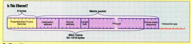
**The Ethernet frame** defines how Ethernet organizes the data in a packet. Hewlett-Packard and AT&T say that the frame defines Ethernet; Grand Junction Networks and its supporters say that the frame is necessary but not sufficient by itself.
