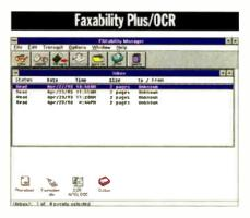
The Intel Faxability Plus desktop opens with the Inbox, a log of received faxes. Across the bottom of the screen are icons for the phone book and the Outbox log, along with an icon for fax-modem status. Faxability Plus lets you customize the view of the Inbox and Outbox logs; you can specify the types of items shown and change the order in which they appear. Faxability Plus doesn't give you the option of printing or viewing faxes on reception; faxes are saved in a queue subdirectory.
