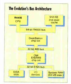
**The Evolution's motherboard** is home for three buses. A 64-bit-wide R4000 bus connects the CPU to a secondary cache: a 486 bus serves as the interface between the R4000 and PC peripherals; and an EISA bus provides expansion. A DeskStation Technology custom chip set links the R4000 to secondary cache and to the 486 bus, while an Opti chip set links the 486 bus to EISA. System memory hangs off the EISA bus.
