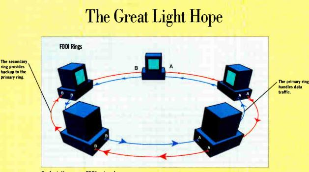
**Each station on an FDDI network** *requires connections to both fiber-optic rings, with the primary ring handling data transmission and the secondary one providing fault tolerance and system management.*
