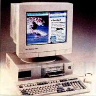
The Image P60 offers PCI support and a 64-bit data path from the Pentium CPU to memory.
