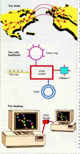
What separates ATM from other networking technologies is its ability to scale from the desktop to the WAN to cable TV to voice networks. Its enormous throughput makes it a strong technology for implementing WANs, and its fast switching makes it ideal as a backbone for interconnecting LANs. It will even show up on some desktops, but only supporting the most data-intensive—and priceinsensitive—applications.
