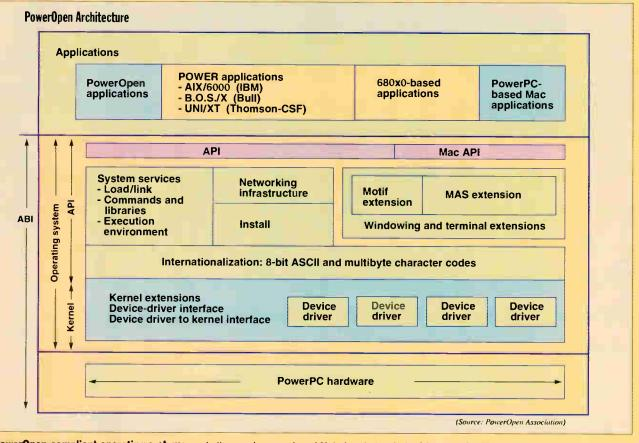
**PowerOpen-compliant operating systems** are built on a character-based Unix foundation derived from IBM's AIX. A common ABI ensures that any PowerOpen application will run on any PowerOpen operating system. OSF/Motif and the MAS are optional extensions. The MAS includes a native Toolbox and a 68040 emulator that support existing 680x0-based Mac applications, and a new generation of PowerPC-based Mac applications.
