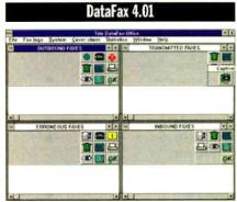
Trio Information Systems' DataFax is composed of five modules. Winserve, the main module, controls the modem and manages the fax traffic. Faxes are either sent in the background or, if Winserve is not running, stored in an outbound queue.
