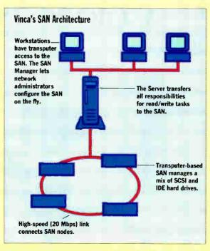
SAN Manager software, which runs on Windows workstations, you can configure your physical storage in practically any number of ways. You can configure a SAN to provide mirroring, data striping, or striping with parity. In fact, you can create any RAID level with SAN software.
