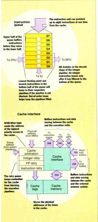
unit can fetch up to eight instructions from the cache during any one tick of the 601's master clock, meaning that the queue can go from empty to full in one clock cycle, assuming a cache hit.
