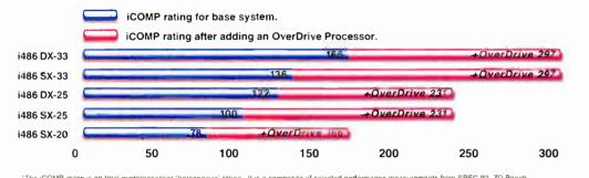
\*The iCOMP index is an Intel microprocessor \*horsepower\* rating. It is a composite of selected performance measurements from SPEC 92, ZD Bench and Whetstone. Source: ICOMP \*: A Simplified Measure of Relative Intel Microprocessor Performance. Intel Corp., 1992
