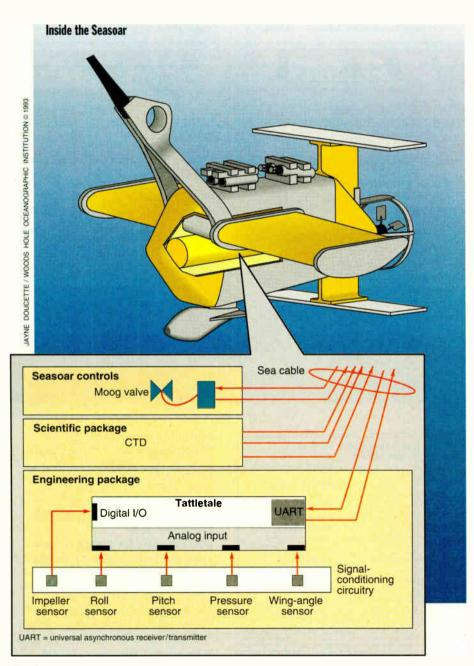
**The Seasoar** contains a control module and two data acquisition components: the scientific package for logging CTD data and the engineering package for determining the Seasoar's status.
