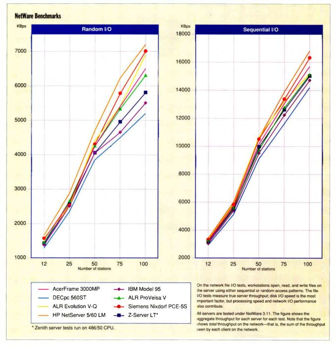
benchmarks don't require hits in main memory. Conversely, the file I/O tests highlight differences in approaches to onboard disk caches as well as to the interface.
