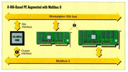
**PC-cluster interface software 0** decouples the CPU from transfer overhead and uses a backplane message-passing protocol, enabling concurrent I/O data transfers at maximum bandwidths. **2** A workstation's ISA bus doesn't have sufficient bandwidth to push data fast enough for I/O-intensive operations. But under applications-software control, a 320-Mbps Multibus II bus can assume I/O-intensive operations. Routine system tasks are left to the ISA bus.
