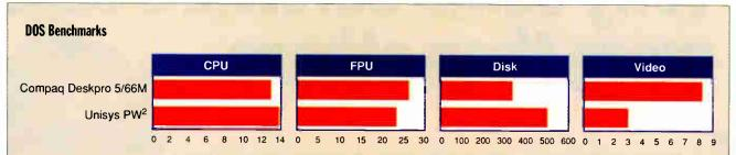
All results are indexed, and higher numbers indicate better performance. For each index in the DOS tests, a Compaq Deskpro 386/33L running Compaq DOS 5.0 = 1.
