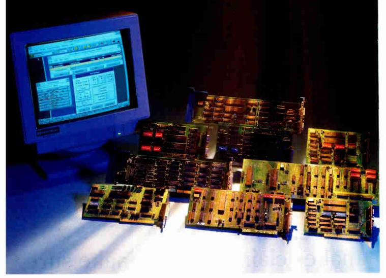
Quatech manufactures a complete line of communication adapters for PC/XT/AT<sup>®</sup>, Micro Channel<sup>®</sup> and compatible buses to meet asynchronous and synchronous, serial and parallel communication requirements with protocols such as RS-232, RS-422, RS-485, Current Loop and IEEE488.
