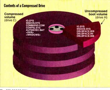
**The DBLSPACE.BIN** kernel file executes from the boot drive immediately after IO.SYS and MSDOS.SYS. Drive C then becomes the CVF, and the boot volume becomes drive H. The latter contains DoubleSpace's hidden files. Note that IO.SYS and MSDOS.SYS are duplicated on the CVF for application program compatibility.
