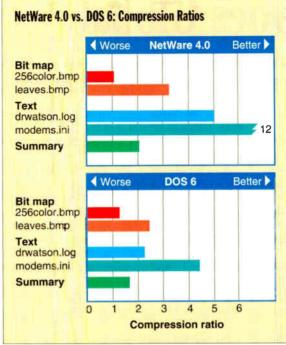
NetWare 4.0 consistently outcompresses DOS 6 on some file types. Results are mixed for bit maps and text files, but on the whole NetWare 4.0 really is a disk doubler. The summary figure represents the composite compression ratio for all files in the Windows directory.
