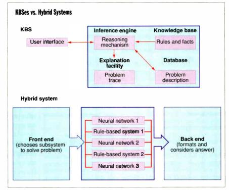
A generic KBS (knowledge-based system) relies on its own database, knowledge base, explanation facility, and inference engine, but a hybrid system can select a subsystem to handle each problem through the front end while the back end formats and consolidates partial answers from each subsystem. (Data courtesy of Silverman, Barry. Expert Systems, Addison-Wesley, 1987; Eberhart, Russell C., and Roy W. Dobbins. Neural Network PC Tools: A Practical Guide, Academy Press, 1990)
