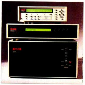
The TAS (Telecom Analysis Systems) Series II modern tester enabled us to re-create 25 telephone-line impairments; this helped us judge how well each modern worked under real-world conditions.
