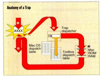
When an exception occurs **()**, program flow jumps to the Trap Dispatcher **(2)**, which uses the Toolbox bit in the trap word to select a dispatch table address. This address is used to locate and execute a routine in ROM or RAM **(3)**. The thread of execution then returns to the next instruction in the Mac program **(3)**.
