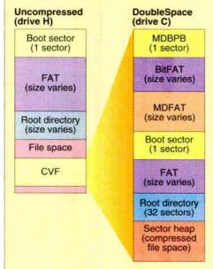
DoubleSpace uses the same data structures as an uncompressed hard drive but adds several new
