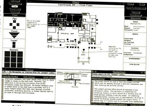
**Archie** is a tool consisting of KBS and CBR technology that provides architectural design support. Here, the system is responding to a request for previous cases pertaining to secure ways of placing people in a courtroom. The floor plan provides two options; a rule is displayed on the bottom right.
