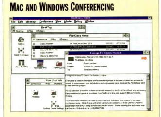
FirstClass Client for Windows (US\$295), a front end for SoftArc's FirstClass E-mail conferencing system, lets clients use a Mac or Windows to access the same nondedicated FirstClass server without need of additional hardware. All connections are over the same Ethernet cable via log-ins over IPX, AppleTalk, and modems. The software accepts up to 250 users simultaneously, allowing Mac and Windows PC users to talk in real time.
