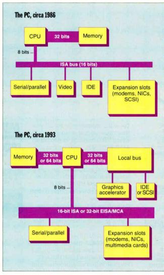
**The trend in PC design** is to move functions off the general-purpose ISA bus and onto wider, specialized buses tied to the speed of the CPU. ISA's 8-bit interface and 8-MHz clock create a bottleneck for all peripheral functions. By contrast, today's systems have 32- or 64-bit paths from CPU to memory and 32- or 64-bit local buses for speedy subsystems such as video and storage. Today's systems also use ISA for slower I/O and to maintain backward compatibility.
