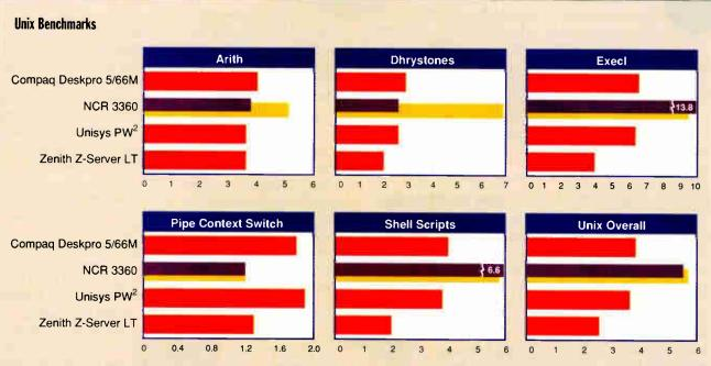
All results are indexed, and higher numbers indicate better performance. For each index in the Unix tests, a Sun Sparcstation IPC = 1. The overall index is the average index of the individual tests.
