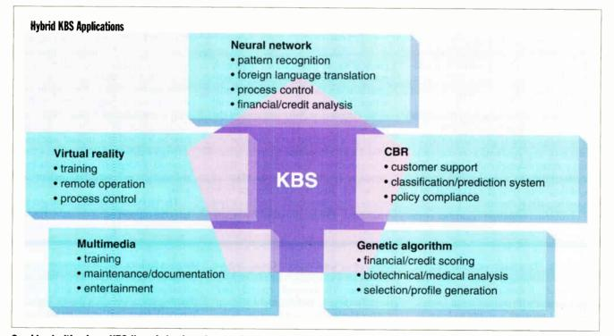
**Combined with a base KBS (knowledge-based system),** such technologies as CBR (case-based reasoning), neural networks, and virtual reality help create applications suitable for a wide range of tasks.
