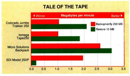
The graph indicates the kind of performance you can expect when backing up and restoring a typical mix of data. The Micro Solutions Backpack was the fastest drive. The SDI Model 250P may have posted better restore times, but its software insisted on scanning an entire tape even after recovering the requested files.
