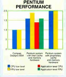
Figure A: Pentium systems can provide nearly twice the performance of a Compaq Deskpro 66M with a 66-MHz 486DX2. One Pentium system, which had its own CPU support circuitry, did better than the other systems we tested. 1.6—again, both compared to a Deskpro 66M with a 486DX2-66.
