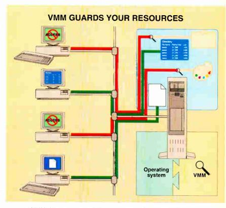
Figure 1: VMMs let you control who has access to files, applications, drives, directories, and servers. The red line indicates that access has been denied. The green line indicates that access has been approved.
