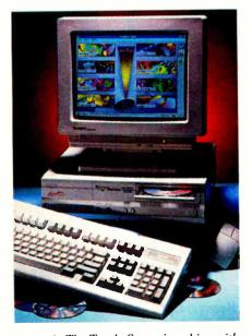
**Photo 3:** The Tandy Sensation ships with an audio adapter, an enhanced internal speaker, a CD-ROM drive, an internal fax modem, and a rich bundle of MPC software and CD-ROM titles. A PC/TV board is optional.
