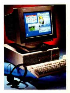
**Photo 2:** An excellent platform for videobased training applications, the NCR 3331 MLS comes standard with Intel's DVI playback board installed. The bundle also includes headphones and a microphone.
