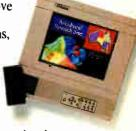
place the Ovation panel on an overhead projector, connect the panel to your computer, VCR, camcorder, or other output device, and you're ready to impress your next audience. Make your presentation even more interactive with the Proxima Cyclops<sup>™</sup> pointer system. It's like a cordless mouse. Point, click, and pull down menus—right from the projection screen.
