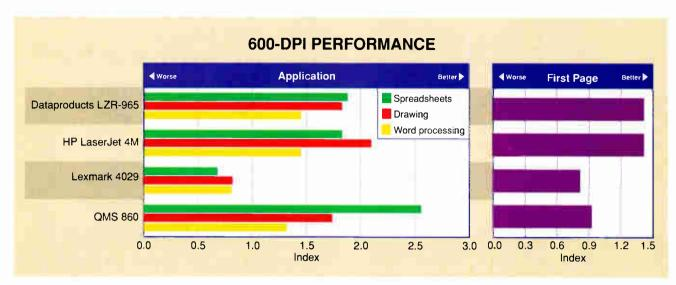
The First-Page Index tests how fast a printer can produce short memos and letters. The Application Index tests common jobs from popular spreadsheets, drawing and design packages, and word processors. Tests are indexed on the LaserWriter IINTX, which has an index of I for each test; longer bars indicate better performance.
