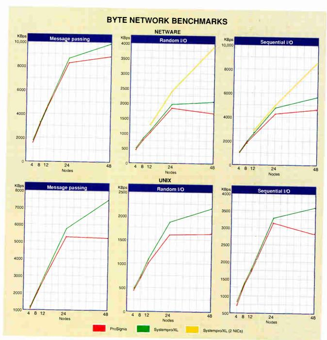
Figure 1: NetWare benchmark results show that both servers are fast but that the Systempro/XL has considerably higher capacity than the ProSignia. The XL shows no degradation at all with two NICs installed. It ran in a dual-processor configuration on the Unix tests, but because I/O is such a significant component of the BYTE Unix Network Benchmarks, the XL doesn't show much benefit.
