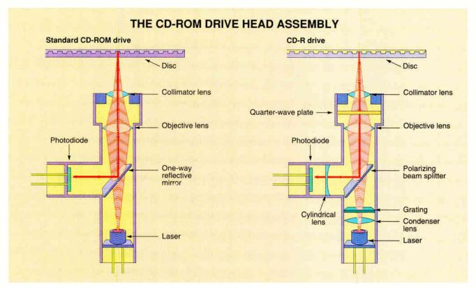
Figure 2: In standard CD-ROM and CD-R drives, a laser beam passes through a one-way mirror or polarizer and a set of lenses on its way to the disc. Reflected light passes through the lenses and is redirected to a photodiode.
