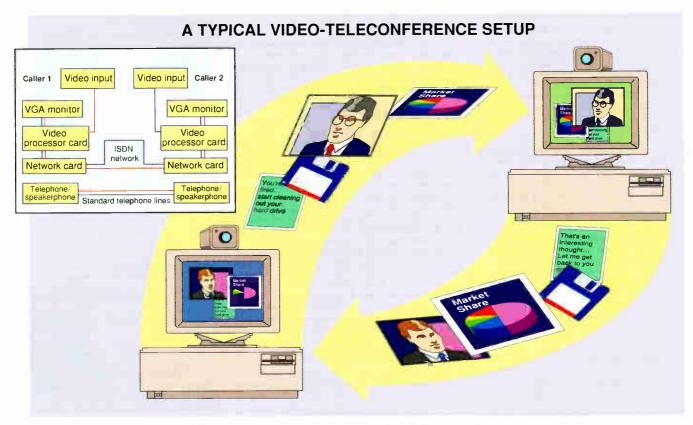
In video teleconferencing, your images are captured by computer-mounted cameras. Video processors digitize and compress images, which are transmitted over a network bidirectionally. Audio travels via telephone lines or through your network.
