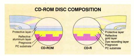
Figure 3: In a standard CD-ROM disc, a manufacturer impresses a pattern of lands and pits into a transparent polycarbonate substrate, which is backed with a reflective aluminum film, a coat of lacquer, and the vendor's label. The drive reads the disc from the bottom, through the substrate. The substrate layer on a CD-R disc is coated with an organic-dye recording layer, a gold layer, and a lacquer coating.
