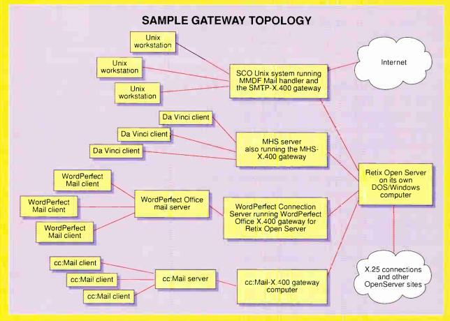
BYTE's network topology, which we used for testing Retix Open Server 400.
