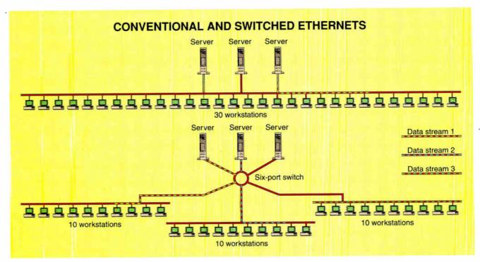
Figure 2: In a conventional Ethernet network with three file servers shared among 30 workstations, only one conversation can take place at a time. With a three-by-three switch added to the network, you can have three conversations on the network at once.
