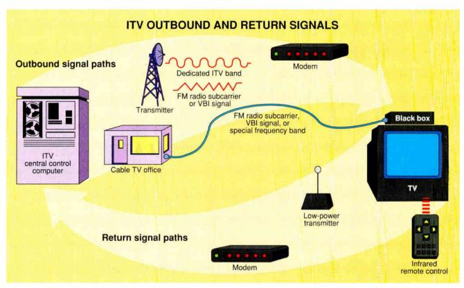
The ITV central control computer transmits signals by FM radio subcarrier or TV broadcast, cable TV, or modem. Your return signals are transmitted via a modem or a low-power transmitter. A black box attached to your TV decodes and encodes signals, and you can program it to scan and store specific information and broadcasts via a hand-held controller.
