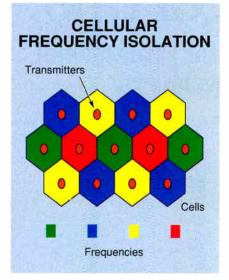
**Figure 1:** In cellular transmissions, the same frequencies can't be used in adjacent cells. Frequencies must be isolated to avoid interference.
