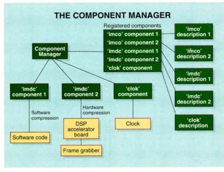
**Figure 3:** The Component Manager functions as a database that classifies objects by function and provides run-time binding to functional objects using the standard Toolbox routines. It allows applications to find predefined classes of software and objects and registers hardware resources. Here, 'imdc' represents the image decompression manager, 'imco' represents the compression manager, and 'clok' represents the system clock.
