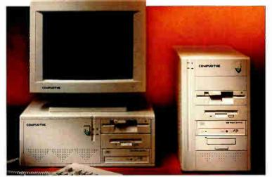
for quick easy upgrades. They support 3 externally accessible 5.25" drive bays and 2 internal 3.5" units.
