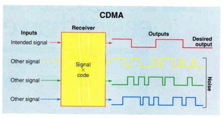
**Figure 2:** With CDMA, all users share the same frequency, but each signal is created with a unique code—the spreading code—that replicates the original signal when multiplied by the signal. As long as the receiver uses the same code, only one signal at the receiving end will decode clearly—that is, as something other than noise.
