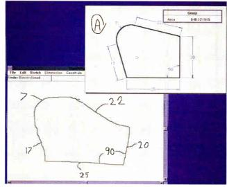
SketchRight by Saltire Software combines a sketch-based drawing package with an embedded Constructive Variational Geometry engine to create a two-way link between the geometry and a mathematical equation solver.
