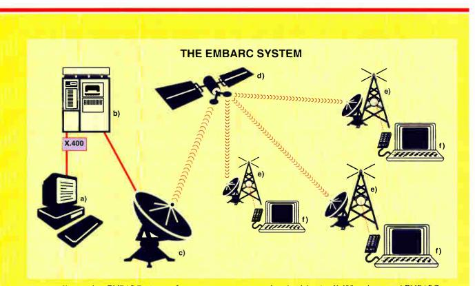
Figure A: You send an EMBARC message from your computer or workstation (a) using X.400 to the central EMBARC switch (b), where a satellite uplink (c) transmits it to a satellite (d). The satellite sends the message to downlink stations (e), which relay them to NewsStream receivers (f).
