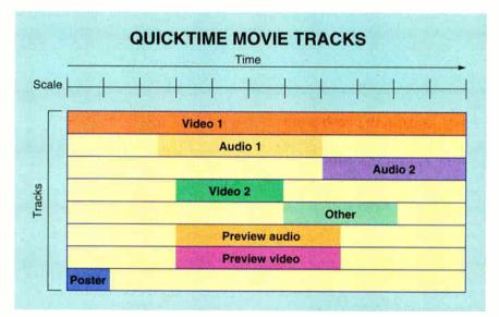
**Figure 2:** A QuickTime movie consists of multiple tracks that reference different data types on various media. Shown are five movie tracks, plus two preview tracks and a poster track. All tracks begin at the start of the movie, although the data does not always start at the beginning of a track. A track can end at any time, and QuickTime plays only those tracks that are active. Multiple tracks can be active at the same time.
