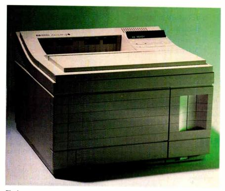
The LaserJet 4M from Hewlett-Puckard includes built-in PostScript and AppleTalk. The new look includes a paper tray that tucks completely into the unit, a more readable control panel, and a true 600-dpi Canon engine.
