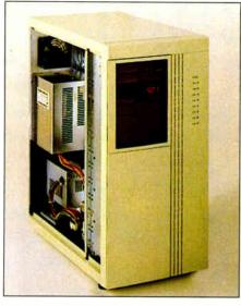
■ Way More Power. With 50 amps of 12-volt power available for start-up, the TP900 easily runs up to 13 power-hungry drives. Perfect for the next generation of super network servers.
