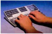
First successful alternative to conventional keyboard saves 60% desk space with a foot print of 27.3 x 15.2 cm. Has full travel tactilly responsive keys with standard left-right spacing for easy touch typing. 100 keys, compatible with IBM XT/AT PS/2. Many language versions available.
