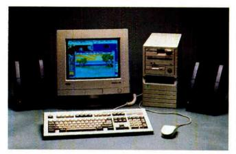
Clover Computer Systems' MPC-1 has real-time window manipulation and a chroma key for overlaying finished live images on a VGA screen.
