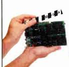
HRT 512-8 ...\$995.00 Real time, grey scale frame grabber. This is a multifleatured high performance industrial model. (LUT, overlay, external trigger, EX./IN. pixel clock, genlockable, optional square pixels, video output...)
