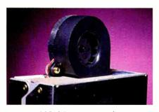
Photo 2: MO drives generate large amounts of heat. Ricoh mounts a small fan on the back of its drive to blow air through the mechanism and out the front of the drive.
