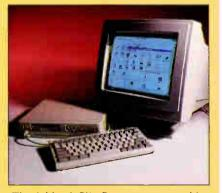
The Addtech SlimPro, a transportable computer similar to the Ergo Brick and the Flytech Carryl, lets you carry your computer from site to site and be able to plug in a full-size keyboard and monitor.
