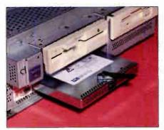
The PC Brand CPU module makes upgrading microprocessors a snap. Inside the cartridge are the microprocessor, coprocessor, cache, and a few support chips. The 9- by 11-inch system board holds the BIOS and main memory, the IDE controller, floppy disk controller, SVGA display adapter, and one parallel and two serial ports.
