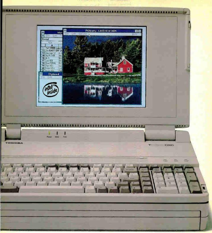
with full-size keys and key spacing, separate numeric keypad and eight dedicated cursor control keys, and nestled it into a compact 11.7 lb. package (12.9 lbs. with color screen). Then attached it to the CPU with a coiled cord, so you can remove it and use it on your lap (or other convenient surface).
