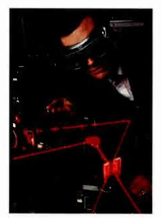
Photo 2: Testing a new polymer that has photorefractive properties. These characteristics may lead to the development of applications such as optical memories or optical data storage many times denser than what is available today. (Photo courtesy of the IBM Research Division, Almaden Research Center, San Jose, CA)
