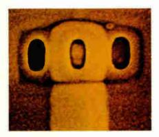
IBM's experimental tiny transistors.
