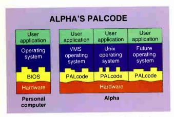
Figure 1: Operating-system independence is the goal of Alpha's PALcode. PALcode consists of subroutines that handle context switching, memory management, and other primitives specific to each operating system. PALcode is similar conceptually to the BIOS of a personal computer.
