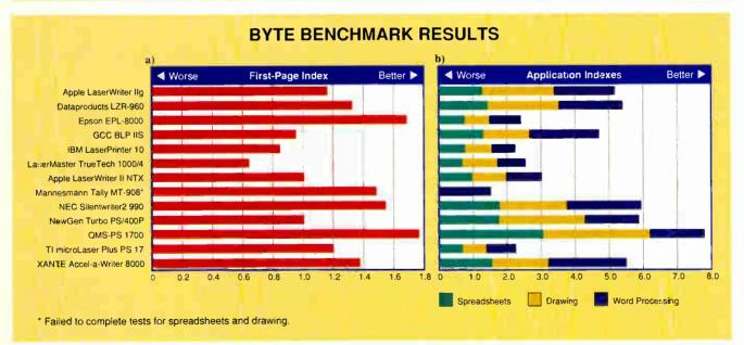
(a) The first-page index tracks each printer's performance on a single page of text, comparing completion time against that of the Apple LaserWriter II NTX. We started timing when the print command was entered and stopped timing when the page fell into the output tray. This test evaluates how efficiently a printer can handle memos and simple business correspondence.
