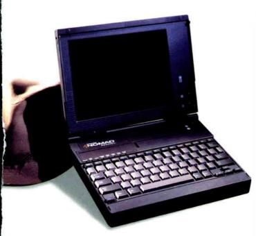
NOMAD Options: 2,400/9,600 bps modems, portable printer, numeric keypad, Token Ring or Ethernet interfaces, SCSI interface, memory upgrades, executive carrying case, extra batteries
