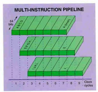
Figure 3: Multi-instruction pipelining requires paying special attention to instruction interaction. In this example of a fourway machine, the instructions E and J cannot execute until the result of A has been computed. However, special bypass logic—a standard architectural attribute—sends both E and J the results of A at the same time the results are entered into the A register, so they don't have to wait an extra cycle.
