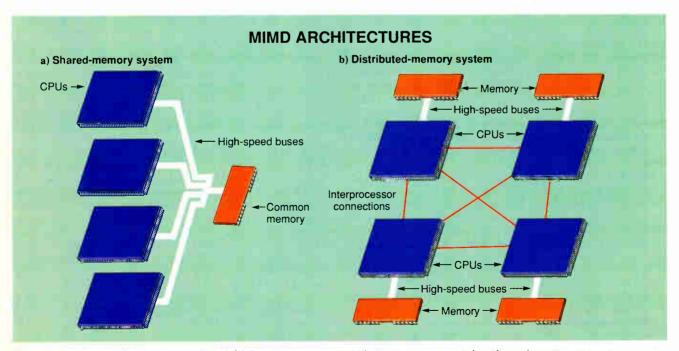
Figure 2: (a) In shared-memory systems, multiple processors communicate over a common bus through a common memory store. (b) In distributed-memory systems, each processor has its own memory store and communicates via high-speed links.
