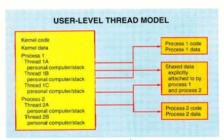
Figure 2: A system providing user-level threads is a protected-memory system in that it protects each process and the kernel, but it allows a process to contain multiple threads of execution. The threads executing within a process have immediate shared access to all global data within the process.
