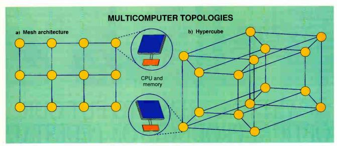
Figure 3: The topology you use in a system depends on the nature of the application. (a) If most interprocessor communication is local—within one or two nodes—a mesh architecture is most cost efficient. (b) When communication is more widespread, a hypercube may be necessary to minimize latency.
