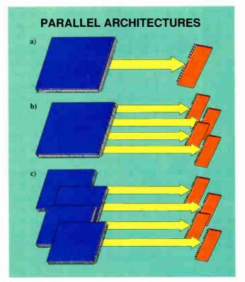
Figure 1: (a) In a serial computer system, one instruction works on one data item at a time. (b) In SIMD machines, many data items are manipulated simultaneously by one instruction or by identical instructions on different processors. (c) In MIMD machines, multiple processors act independently on different data items.
