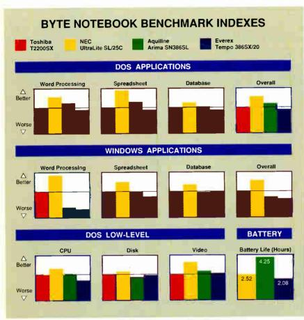
All results are indexed, and higher numbers indicate better performance. For each index in the DOS and Windows tests, a Toshiba T2200SX running DOS 5.0 and Windows 3.0 = 1.
