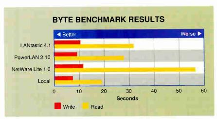
LANtastic 4.1 comes close to toppling PowerLAN 2.10, the fastest peer LAN we've tested. The newest LANtastic also easily outguns Novell's NetWare Lite. Local tests (timed directly on the host machine) are included for comparison.
