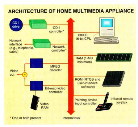
Figure 1: The architecture of a home multimedia appliance has most of the same components as a low-end PC, with digital video and audio decoders added. The CPU and RTOS manage the flow of data from the optical disk or network interface to the decoders and run the GUI.
