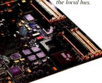
Photo 2: The motherboard in the Vectra 486u has a second socket to implement Intel's overdrive scheme.
