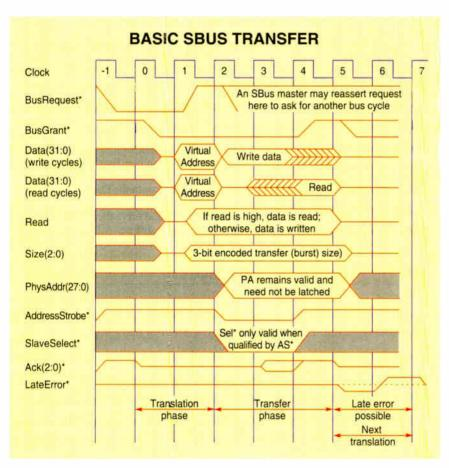
**Figure 3:** During arbitration, SBus masters request and are granted access to the bus. The translation phase converts virtual addresses to physical addresses. Then, in the transfer phase, data moves between master and slave. Arbitration occurs in parallel with translation and transfer, between clocks -1 and 0, and again between 2 and 6.
