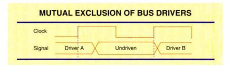
**Figure 2:** Driver A is disabled on one clock edge, and driver B is enabled on the next. This ensures that no more than one output will drive a signal during any clock cycle.
