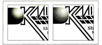
Figure 1: The 400-dpi WinPrinter produces noticeably smoother gray scales and crisper line edges (left) than do 300dpi printers like the Hewlett-Packard LaserJet (right).
