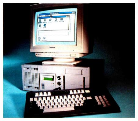
The front panel of the FTSA PC provides diagnostics messages through the LCD and access to redundant power supplies and disk drives.
