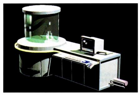
By reflecting lasers off a rotating mirror, Omniview creates a series of 2-D images, which your eve fuses into 3-D shapes. (Courtesy of Texas Instruments)
