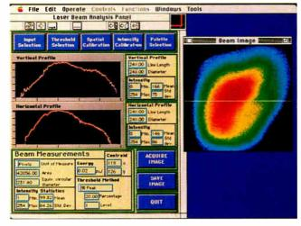
Beam Analysis Vi monitors multiple laser beam characteristics simultaneously.
