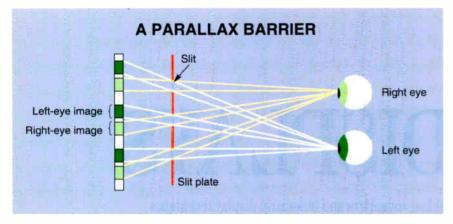
**Figure 1:** This cross section of a parallax-barrier system, seen from above, shows how the system sends different images to each eye. When you are the proper distance from the slit plate, each eye sees only the image strips meant for it. The slit plate occludes information meant for the other eye.
