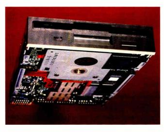
track pitch. Floptical uses closed-loop servo-positioned heads that read rings that are preprinted on special disks. The result is that Insite can cram 1245 tracks per inch onto the medium, compared with 45 to 135 tpi for floppy disks. The linear density is higher, too, at nearly 24,000 bits per inch (versus 17,000 bpi for high-density drives).
