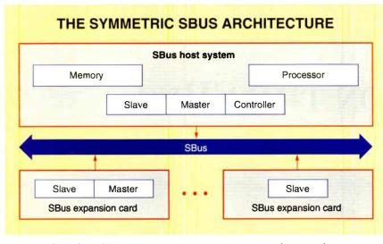
**Figure 1:** Every SBus has one or more masters, one or more slaves, and one controller,
