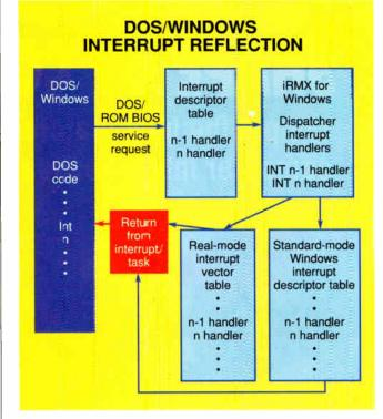
Figure 4: Any iRMX task. including DOS/Windows, can initiate hardware interrupts. The system traps DOS/Windows interrupts in Ring 0; reflects them to the appropriate handler, whether real-mode or protected-mode; and then traps the return to route the tasks to the appropriate mode.
