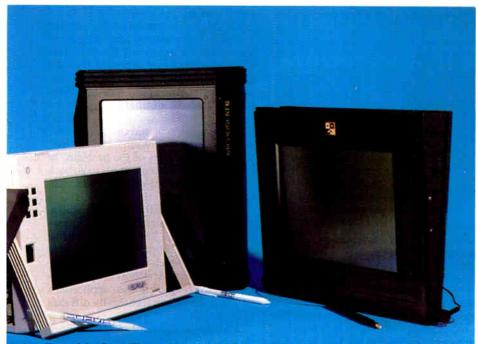
Five of the first: These pen-input machines, ideal for mobile-computing applications, represent the first generation of pen-based systems. From left to right: the TriGem Pen386SX, the GridPad HD, the DFM Systems TraveLite, the MicroSlate Datellite 300, and the Momenta Computer.
