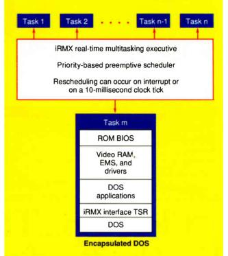
Figure 2: DOS runs as an iRMX task like any other in V86 mode. The DOS task contains a normal DOS system complete with drivers, ROM BIOS, and applications. In that same iRMX task, you can initiate Windows just as you would on a dedicated DOS system.
