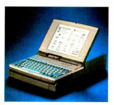
**Photo 2:** The docking station is almost as portable as the notebook itself. It weighs only 9 pounds with its batteries.
