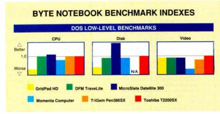
Low-level benchmark results for pen-input systems. The 20-MHz 386SX-based TriGem and Datellite systems did well, but there was relatively little variation. The Momenta Computer scored poorly, with low scores on memory-move tests. Toshiba's T2200SX is included as a baseline for comparison.
