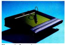
**Momenta Computer** The "pentop" Momenta Computer is interesting and innovative, designed for both desktop and mobile use. With the keyboard attached, you can tilt the display and use the computer as a desktop, or you can operate it with a pen without the keyboard. However, the Momenta weighs in at over 6 pounds, making it heavy for extended hand-held use. The machine measures 10 by 12 inches and is wedge shaped, making it a bit bulky for the crook of the arm.
