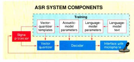
**Figure 2:** The components of an ASR system work in synchrony to produce the best possible interpretation of speech input.
