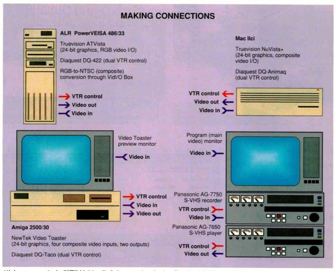
All three systems in the BYTE Multimedia Lab are equipped to handle video I/O. The end of the line is always the video input of the AG-7750 S-VHS VCR. If only the real interconnections were as neat and manageable as in this diagram.
