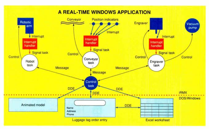
**Figure 1:** The top part of the figure details the real-time components of a luggage-tag engraving application, including control tasks and hardware interrupt handlers. The bottom part shows a Windows screen (e.g., an Excel window for order entry, a custom window showing the control system graphically, and a soft-control panel), which might conceal the control system at the top. The iRMX for Windows operating system establishes the linkages to accomplish this on a PC.
