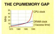
**Figure 2:** The curves representing clock speed and memory speed have diverged markedly since the introduction of personal computers in the mid-1970s. This divergence points out the need for caches and other bandwidth-expanding techniques that let memory systems keep up with modern processors.
