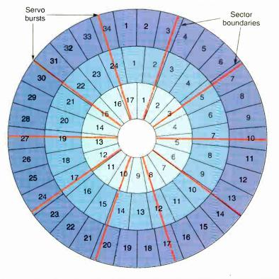
**Figure B:** *CDR is a more efficient storage method that is now gaining acceptance. It breaks each disk platter into concentric zones, each with a recording density optimized for it. Because the outer zones are larger in circumference, they can contain more bits. More sectors are recorded in the outer zones than in the inner zones (cach sector contains the same number of data bits).*
