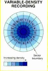
Figure A: Typical hard disks have used variable-density recording, which writes data at a constant rate to a disk rotating at a constant angular velocity. Variable-density recording results in a lower density (and lower storage efficiency) for recorded data on the outer tracks of a disk. the outer zones than in the inner zones in the same amount of time (the motor speed is constant), the data rate is higher in the outer zones. This method is called *constant-density recording* (see figure B).
