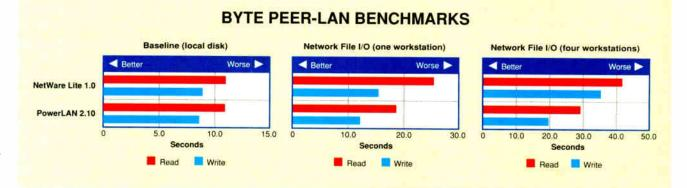
NetWare Lite is fast, but not fastest. PowerLAN, the fastest peer LAN BYTE has tested, outran NetWare Lite on our tests. NetWare Lite's score of about two-thirds the speed of PowerLAN makes it about average among peer LANs we benchmarked in November.
