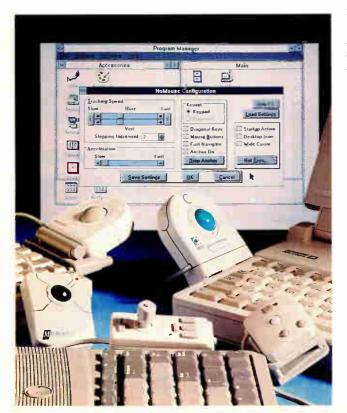
Photo 2: A litter of mice and mousealikes: the Abacus NoMouse for Windows (screen); clockwise from right: the Logitech TrackMan Portable, Appoint Thumbelina Portable, Suncom ICONtroller, **MicroSpeed** MicroTrac, and Microsoft BallPoint Mouse.
