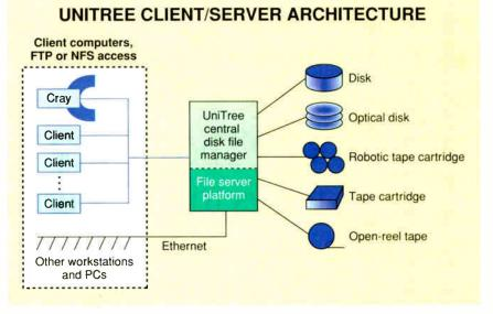
**Figure 2:** UniTree from the Discos Division of General Atomics provides automatic and transparent file and storage management for Unix networks that use NFS or FTP access. Shown here in its simplest form, UniTree is being enhanced with software modules that run on client computers to form what the company calls a Virtual Disk System, whereby files are invisibly migrated from a client or server disk further down the storage hierarchy.
