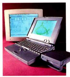
Photo 2: The PowerBook 100, with an Envisio memory/video expansion board. Envisio's Notebook Display Adapter is driving a second screen on the AppleColor 13-inch monitor in the background while providing an extra 2 MB of RAM.
