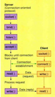
The typical flow of events for a connection-oriented transfer using sockets. (Figure courtesy of Unix Network Programming by W. Richard Stevens, Prentice-Hall, 1990.)
