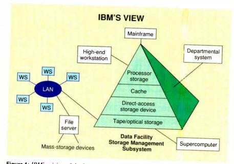
**Figure 1:** *IBM's vision of the future for what it calls system-managed storage is based on its Data Facility Storage Management Subsystem. The near-term extensions will be to clients and servers running under IBM's AIX and OS/2 and under SunOS, for uploading to an MVS/ESA computer for backup and archiving.* (WS = workstation.)
