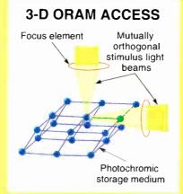
Figure A: 3-D ORAMs record information through the excitation of a photochromic chemical dopant. To read a bit, two photons of 1.03-micrometer wavelength provide the necessary stimulus when they strike a data bit.
