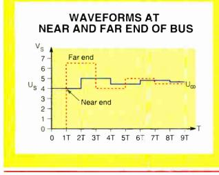
Figure B: A logic transition occurs at the near end of a bus at time 0 and arrives at the far end at 1T, with significant overshoot. The overshoot propagates back to the near end and changes the voltage there. The reflections travel up and down. decreasing, until at 8T the bus settles near its final logic level.
