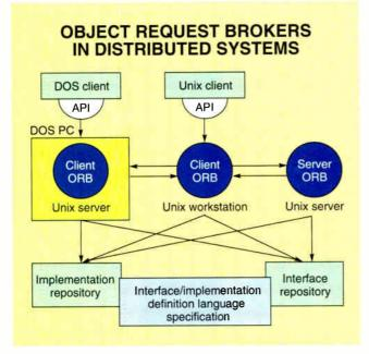
**Figure 1:** The Object Request Broker is the kernel of a standardized DOMS and provides interoperability and reuse of a system's existing objects. The ORB enables client applications to access services and other objects that exist anywhere in the distributed system.
