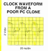
Figure C: This oscillograph is taken from an early ISA clone. It shows the system clock (pin AXX) measured at the end of the bus and severe overshoot. directly, without any series-damping resistor. The output impedance of this buffer (which should be greater than  $Z_{ff}/2$  to control overshoot) is extremely low when the signal goes from high to low (the *pull down* cycle) but fairly high when the signal goes from low to high (the *pull up* cycle).
