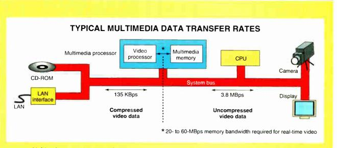
Figure A: Multimedia processing moves data over the system bus in both compressed and uncompressed formats. The values given here are typical for one-way transfers on a single video stream. Applications such as video conferencing will require the system to simultaneously handle two streams of video information, doubling the bus traffic shown here.
