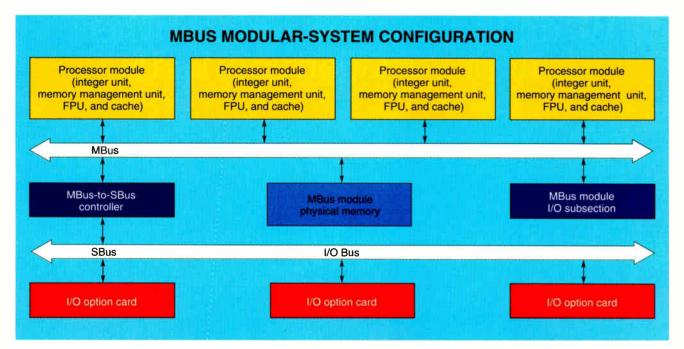
Figure 4: MBus is a SPARC module interconnect bus that supports symmetrical multiprocessing for as many as eight processors and provides data transfers as high as 320 MBps. Systems using MBus as a processor bus also use a separate I/O bus, such as the SBus shown here. The MBus protocol includes the cache-coherency logic necessary for SMP operations.
