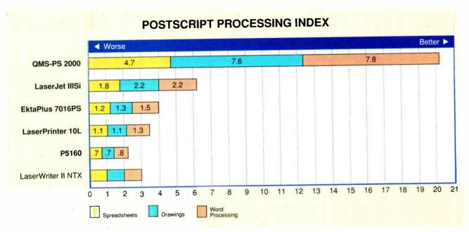
The BYTE PostScript test suite, which was built on industry-standard tests created by Genoa Technology, compares PostScript capabilities running spreadsheet, drawing and illustration, and word processing applications. Within the primary printer group, the LaserJet IIISi prevailed in each category. All results are indexed to the Apple LaserWriter IINTX (which equals I for each test). Longer bars indicate better performance.
