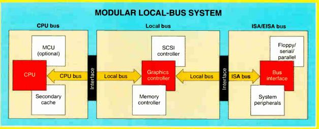
**Figure A:** This three-layered system uses a modular local bus running at 33 MHz to interconnect speed-critical functions. The system now supports 486 CPUs at speeds of up to 100 MHz and provides connections for slower peripherals on a standard 8-MHz ISA bus. The key element of the system's architecture is the separation of the CPU bus from the local bus; other architectures may connect the CPU directly to a local bus.
