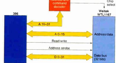
Figure B: The extended-math-coprocessor interface used by Cyrix and Weitek transfers data and commands over the data bus and the address lines.
