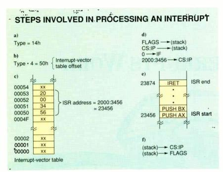
(a) Type byte received: type 14h; (b) multiply type byte by 4 to get interrrupt-vector table offset (50h); (c) get ISR address (2000:3456) from interrupt-vector table (location 00050h); (d) push FLAGS register, Code Segment, and Instruction Pointer onto the stack, clear the interrupt-enable flag (IF), and branch to the ISR; (e) execute the ISR (at location 23456h), terminating with an IRET instruction; and (f) restore Instruction Pointer, Code Segment, and FLAGS register from stack.
