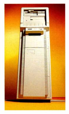
he company that has made a decent living challenging Compaq has now introduced its rival to the Systempro. The EISA-based Dell 433SE packs a 486 microprocessor running at 33 MHz and the newly released Dell Drive Array (DDA). The system shipped to BYTE (with 16 MB of memory, four 200-MB IDE hard drives, and an optional tape drive) sells for \$12,998, a bargain in this market.
