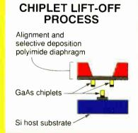
Figure A: The GaAs devices on the polyimide diaphragm are aligned with respect to the silicon host substrate, and they are deposited from the diaphragm onto the silicon. Individual devices or an entire array of devices can be aligned and deposited onto this host substrate.
