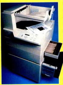
Based on a 25-MHz Mips R-3000 takes networked printing to a level beyond typical 10- to 20-page-per-minute printers. For example, the QMS-PS 2000 ran through the entire PostScript test suite three times faster than the next best printer.
