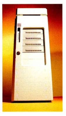
angent has added a formidable competitor to the file-server market with its 486-based Multi-Server. The processor runs at 33 MHz and takes advantage of a standard 256-KB SRAM cache. Although the Multi-Server can use only a single CPU, it addresses the I/O bottleneck issue elegantly with the powerful combination of EISA bus mastering and a SCSI-2 interface. The unit we received carried 16 MB of memory, four 165-MB SCSI drives, two SCSI controllers, and a price tag of \$14,500.
