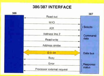
Figure A: The Intel 386/387 coprocessor interface transfers data only over the 32-bit data bus.
