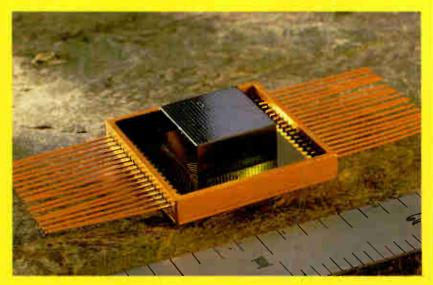
**Photo A:** One three-dimensional IC, such as this cubclet from Irvine Sensors, stacked 92 memory ICs of 4 Mb of DRAM to create a 40-MB package.
