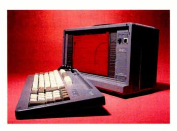
The 486-50E comes standard with a Conner Peripherals 200-MB SCSI hard drive and a 3½-inch 1.44-MB floppy drive. There's no room to add further storage, but you can buy the machine with a larger hard drive. I found the 200-MB drive and the 4-MB caching controller to be an effective combination.
