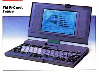
The Fujitsu FM R-Card fits in a briefcase and offers the features of a desktop machine. It weighs only 2.2 pounds, measures 11.6 by 8.3 by 1.04 inches, and has a full-size, keyboard. It runs for 8 hours
