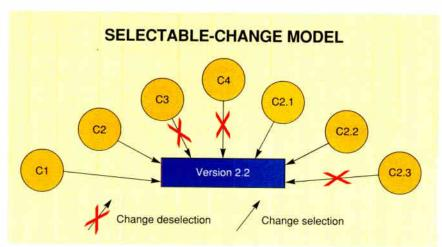
Figure 2: The circles indicate changes. A version specifies a collection of selected changes. The diagram shows the change selections for V2.2 shown in figure 1 as though a single logical change were made between the versions.
