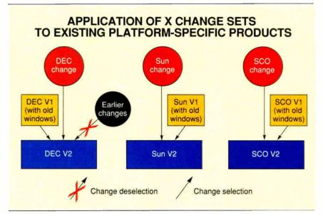
Figure 4: A new version of the products built using X features results from the application of the change sets to the existing version of each of the products.
