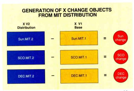
Figure 3: A change set results from the difference between an existing version of the X files for each platform and the updated files provided in the MIT distribution version for that platform.
