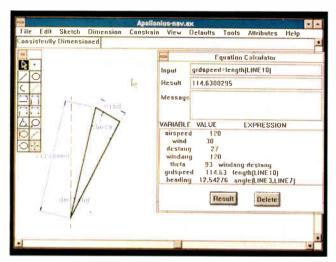
Apollonius for Windows 3.0 can solve geometry problems without requiring you to remember formulas. The program offers a sketch-based drawing package and a variational geometry solver.
