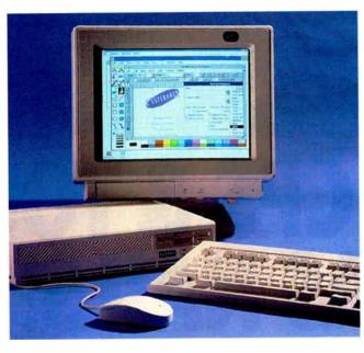
top-of-the-line model. It includes 32 MB of RAM, a 3%-inch 426-MB SCSI hard drive, an 8514/A graphics card with integrated VGA and support for 1024- by 768-pixel noninterlaced resolution, 1 MB of video RAM, and a 15-inch Super VGA color monitor.
