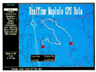
RealTime MapInfo integrates with technologies such as the Global Positioning System to track the exact location of moving objects on electronic street maps. A GPS processor takes readings from three or more satellites to determine longitude and latitude. Then a vehicle equipped with a GPS receiver sends its position to a receiving station via serial port, cellular phone, or hard connection for geographic display on RealTime MapInfo.
