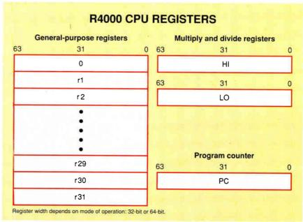
Figure 1: Only two of the R4000's registers have special functions: Register 0, following RISC convention, is a bit bucket, and register 31 gets the return address during subroutine calls. The multiply and divide registers store the 64- or 128-bit results of integer multiplication operations or the quotient and remainder of integer division operations.
