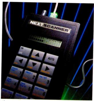
After testing network wiring, Next Scanner compares the results to a table and indicates if the cable will support the application.
