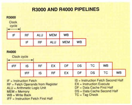
Figure 3: The R4000's eight-stage pipeline advances twice per clock cycle; the R3000's five-stage pipeline advances once per cycle. A superpipelined processor requires less silicon and less logic design effort than a superscalar processor. But since superpipelining depends on fast logic, circuit design is tougher. And since the pipeline can be split into only so many stages, the approach eventually runs out of steam—at which point the designers must contemplate a superscalar design.
