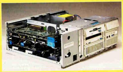
With the addition of a DVI-based ActionMedia II board, the system can provide playback of digital video applications.
