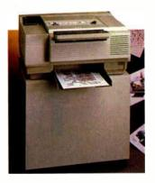
The Phaser III PXi's intelligent multitasking interface has automatically switchable parallel, serial, and AppleTalk ports. The print area of the Phaser III PXi can be as large as 12 by 18 inches, permitting full-size 11-by 17-inch bleeds.
