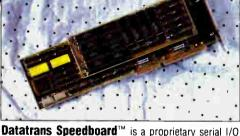
controller, developed by Datatrans to handle heavy data transfer in a multiuser computing environment. With its on-board 16 MHz 80186 processor, up to 512 KB of memory buffer, and statistical supporting software. Speedboard relieves main CPU overhead and effectively accelerates I/O speed.
