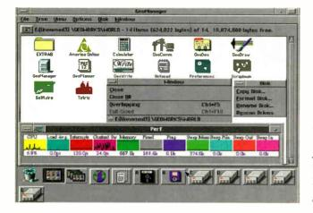
a screen-capture utility, and Perf-a set of performance gauges that dynamically display what's happening in the system. Also included are a couple of demonstrations that eat up CPU time. Nevertheless, the system just keeps zooming along. It's a heck of a display of Ensemble's multitasking capabilities.
