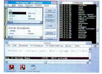
File Express displays the local C drive and a remote directory on a CompuAdd SS-1. In a DOS window, a listing of the local F drive shows files on a Swan PC running Interactive Systems' Unix, thanks to BW-NFS. The Unix mail reader elm runs in a Host Presenter session connected to the Swan. Additional Host Presenter sessions connected to other Unix hosts run as icons, as does Serving FTP, Novell's File Transfer Protocol server for Windows.
