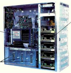
Hot Plug ™ drives. If any one of the five drives fails, the IAS will automatically rebuild the data on the replacement drive, while continuing to respond to I/O requests from the host.
