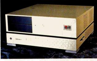
Texas Microsystems' SBus Expansion Box increases Sparcstation capacity. The 9100 is compatible with all DMAcontrolled SBus cards, according to the company.
