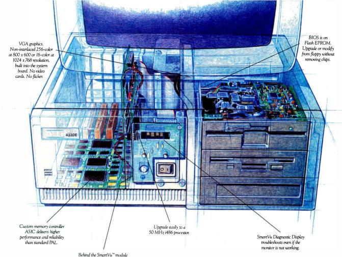
Behind the SmartVu<sup>™</sup> module lie industry standard SIMMs so extra memory can be added easily and inexpensively.
