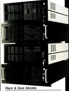
Accepts PC, XT, AT Motherboards and Passive Backplanes Doesn't Look Like IBM Rugged, Modular Construction Excellent Air Flow & Cooling Optional Card Cage Fan Designed to meet FCC 204 Watt Supply, UL Recognized 145W & 85W also available **Reasonably Priced**
