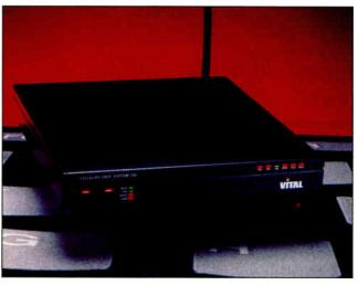
The external status indicators of the Cellular Data System 120 keep you abreast of important information, such as low battery power, roam, lock, no service, and test.
