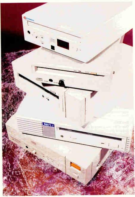
Third-generation CD-ROM drives offer data-access times of 350 ms or better and entrance to an ever-widening world of databases. The six drives tested are built by (from top) Chinon, Texel, Toshiba, PLI, and Hitachi.
