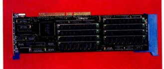
The self-configuring OS/RAM32plus provides up to 128 MB of extended and expanded memory in one slot.
