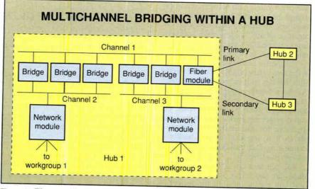
Figure 5: The use of bridges within a multichannel hub provides fault tolerance and, using a spanning tree, congestion control. No module will be isolated if any bridge fails, and the failure of any channel will not affect the workstations on the other channel.
