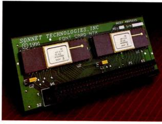
Sonnet's FontCard NTX increases the LaserWriter IINTX's capabilities.
