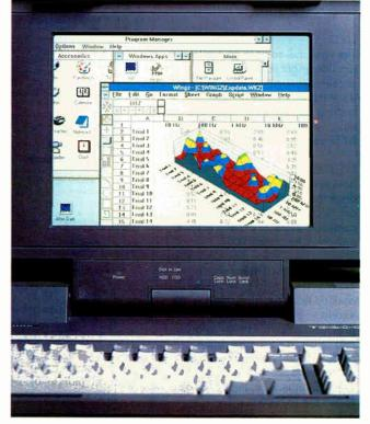
**Photo 2:** The Toshiba T3200SXC's display is simply gorgeous. The backlit LCD, based on active-matrix technology, responds quickly enough to keep up with a mouse cursor.
