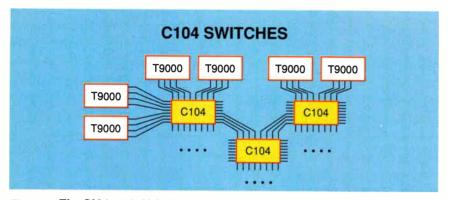
Figure 3: The C104, with 32 links, can route 16 simultaneous conversations. It uses worm-hole routing and has a switching latency of just 700 nanoseconds.
