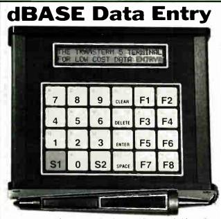
The TransTerm 5 is a work station data entry/display terminal for on-line shop floor data collection into PC/AT based systems. The unit is one of a family of such terminals which feature LC displays for operator prompting and data entry via a membrane keyboard or an optional barcode wand (Code 39). A multi-terminal polling controller (up to 250 stations) and a dBASE III + compatible software package are also available. System costs below \$300.00 per station. Call for info.
