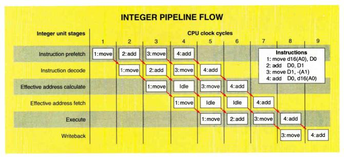
Figure 2: Each of the instructions will occupy a pipe stage for only one clock cycle; therefore, one instruction can complete in each clock cycle.
