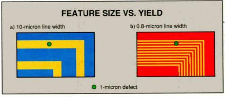
**Figure 2:** Whether a wafer defect constitutes a flaw in a chip depends on the feature size. A chip with 10-micron metallization line width will be essentially unaffected by a 1-micron open-circuit flaw (a), whereas the same defect will kill a chip with denser circuitry (b).
