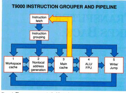
Figure 2: The grouper automatically fills the five-stage pipeline.
