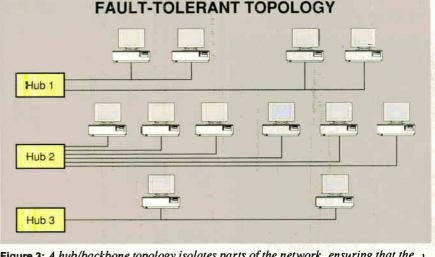
**Figure 3:** A hub/backbone topology isolates parts of the network, ensuring that the stallure of one module will not affect all the rest. The higher the ratio of modules to workstations, the greater the fault tolerance of the network as a whole.
