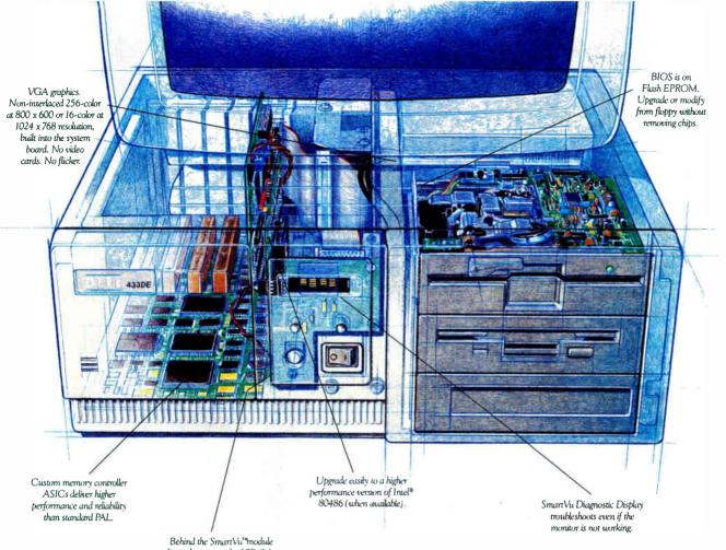
Behind the SmartVii<sup>™</sup>module lies industry standard SIMMs so extra memory can be added easily and inexpensively.
