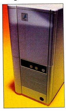
he FlexComServer 100 is a plugand-play alternative to installing processor cards on your LAN. It consists of a 16-MHz 286 system bundled with Cubix processor cards, a network card, a floppy disk drive, and all the software you need to get a dial-in system up and running. Evergreen Systems also bundles a copy of DMA's pcAnywhere IV/LAN remote-control software. I tested the FlexComServer 100 (\$2195) with two Cubix CP-2286 dual-286 processor
