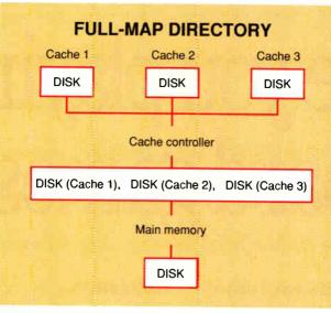
Figure 1: In a full-map directory, every cached block has a record and a pointer in the cache controller. The record includes status flags that indicate whether you can write to the block and whether it is a valid block. The costs for a centralized cache directory are primarily memory overhead, more controller processing demands, and communications bottlenecking.
