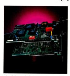
The Twincom 24/96 uses the Rockwell RC9624 chip set.
