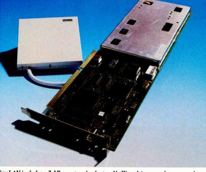
WaveLAN includes a 2-Mbps network adapter, NetWare drivers, and an external antenna (upper left).
