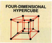
Figure 4: A four-dimensional hypercube has the logical structure of a tesseract. It has 42 processors, each with connections to four other processors. The communications diameter is 4.
