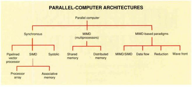
**Figure 1:** Ralph Duncan's classification of parallel architectures provides a common vocabulary for discussing parallel computing. Multiprocessors are synonymous with Duncan's MIMD classification.
