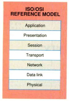
The seven layers of the OSI model for networks are designed to make the specification endure many changes in technology. StarLAN, ARCnet, and X.25 networks.
