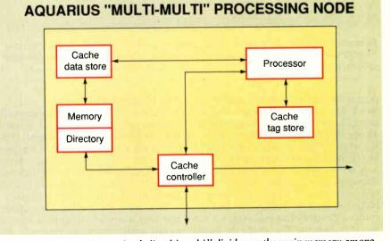
Figure 2: The Aquarius project's "multi-multi" divides up the main memory among the processing nodes and adds a directory scheme to a snooping scheme to ensure cache consistency.
