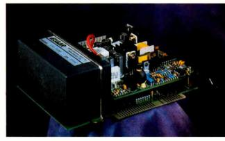
Intelligent Power System on a Card provides on-line battery backup for your PC or workstation.
