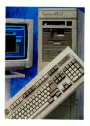
model sports three half-height front access and two half-height internal 5.25" drive bays, six 16-bit and one 8-bit expansion slots. So
