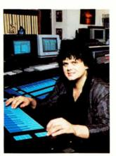
The Atari Hotz MIDI translator, although resembling a keyboard, is completely programmable and doesn't have any moving parts. The pads are touch-sensitive.
