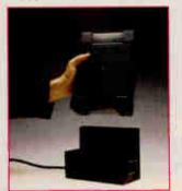
port allows easy, drop-in connection to our Docking Terminal, \$349, which instantly hooks up all cables and provides another 16-bit 3/4 length slot. The "Stretch" version of the Brick accomodates full length cards.
