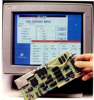
Optoelectronics PC-10 Universal Frequency Counter uses Windows 3.0 for instrument control.
