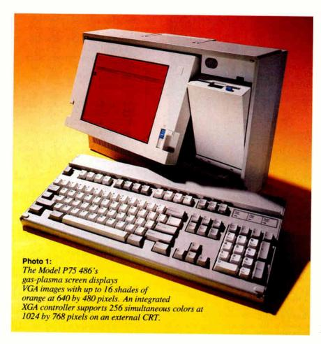
ost of the new powerful 33-MHz 486 systems come in large desktop or tower cases, but faster doesn't have to be bigger. IBM's PS/2 Model P75 486 portable proves that point.
