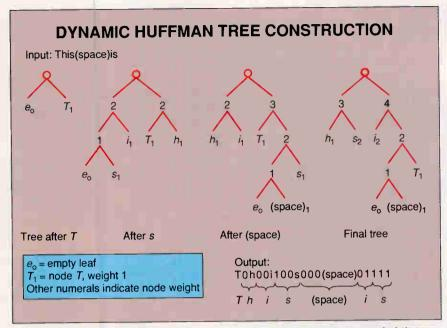
The Huffman encoding tree changes to respond to changing character probabilities in this dynamic example. At first, all the transmissions are empty leaf code/literal character combinations. When i and s are transmitted a second time, the compressor uses their codes instead of literals. As s is reused, it moves higher up the tree, shortening its corresponding code.
