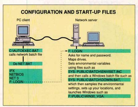
You should plan on having some configuration files on the server, and others (as shown) on each client machine. Each configuration and start-up file has an appropriate location.
