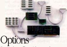
Our products offer serial port and memory options that are field upgradable; compatibility with ISA (AT), MicroChannel and EISA buses; RS232, 422, 485 and Current Loop interfaces and DB 9, DB 25 and RJ 45 connectors.
