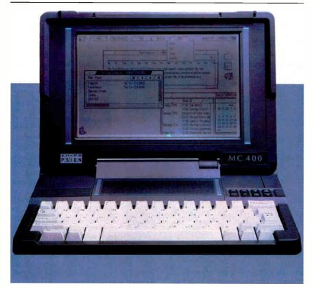
Photo 2: Psion's MC400 laptop incorporates a touchpad that lets you "point and drag" with your fingertip. The touchpad's aspect ratio is different from the screen's; it had to be squeezed in above the keyboard, so its horizontal resolution is about twice its vertical resolution.
