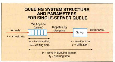
Figure 2: Shown here are the queuing system structure and parameters for a single-server queue. The central element of the system is a server. If the server is idle, an item is served immediately. Otherwise, the item joins the queue. When the server has completed serving an item, that item departs, and the next item (if there is one in the queue) is immediately dispatched to the server.
