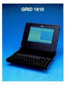
The 1810 doesn't have the black magnesium case that's become a Grid trademark, but it has the same rugged feel and some interesting features. Powered by an NEC V20 microprocessor, the Grid 1810 posted performance numbers in the same range as the XT-class notebooks. Unfortunately, the 1810's battery life doesn't measure up to that of the other machines in its class.
