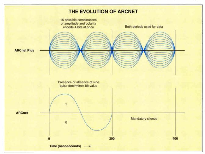
The original 2.5-Mbps ARCnet signals bit values by determining the presense or absence of a sine pulse. Here, ARCnet signals a "1" bit by sending a 200-ns pulse, followed by a silence of equal length. The 20-Mbps ARCnet Plus specification makes more efficient use of the bandwidth by using both periods for data and by using amplitude modulation to encode 4 bits into every pulse. ARCnet Plus also sends a calibration pattern once for every 8 bytes, further reducing overhead.
