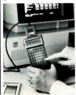
display, several different keyboard designs, and from 32K to 96K of internal RAM memory. All Organiser units can use our removable and interchangeable memory modules, allowing the Organiser II to be configured to meet your unique data and program memory requirements.
