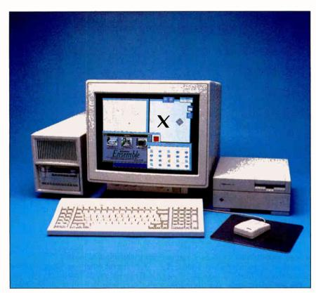
Photo 1: The Sparcstation IPC's tiny case is just large enough to hold up to 24 MB of RAM, one 3½-inch SCSI hard disk drive, one floppy disk drive, and two SBus expansion cards. The taller case is the expansion unit, housing a SCSI hard disk drive and a tape drive.
