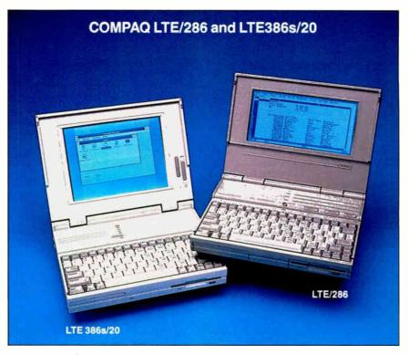
oth of the Compaq notebook machines bear a striking family resemblance, but beneath the exterior, the LTE 386s/20 has a completely new design that incorporates Intel's 20-MHz 386SX. The LTE/286 uses a 12-MHz 80C286 processor. Both accept a math coprocessor and include floppy and hard disk drives. The 386s/20's 2.2-inch-high case—which is slightly thicker than the LTE/286's case—makes that notebook the tallest machine in the group. Both Compaqs are relatively light and easy to carry.
