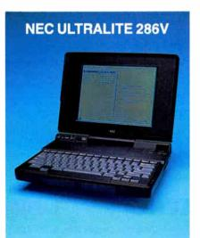
The UltraLite 286V keyboard has one of the best layouts of the machines we tested; it has large Enter, Shift, Control, and Alt keys and separate cursor-control keys. But the short, 2-mm key travel may annoy some touch-typists. The keyboard also doesn't offer much tactile feedback.
