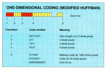
Figure 3: In one-dimensional coding, the sender looks for transitions from black to white (or vice versa) and reports the number of pixels since the previous transition. To prevent an unsightly blotch from appearing in the event of an error, the line must always start with a "white" run length (which can be zero if the first pixel is black, as shown above). The code for a run of black pixels is not the same as for an equal number of white pixels because they are not as statistically likely.
