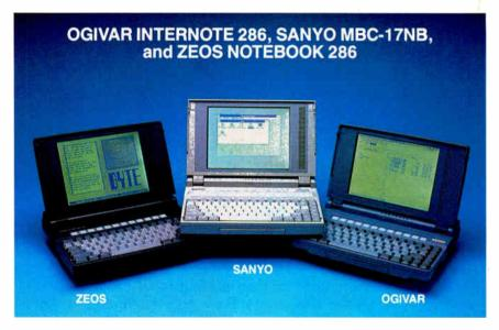
The units fold into a compact 7-pound shell. All three appear to be solidly constructed, durable machines. A row of indicator lights lies on the main unit, just below the screen, remaining visible when the screen is folded down. A handle pops out from the front of the unit for easy carrying.
