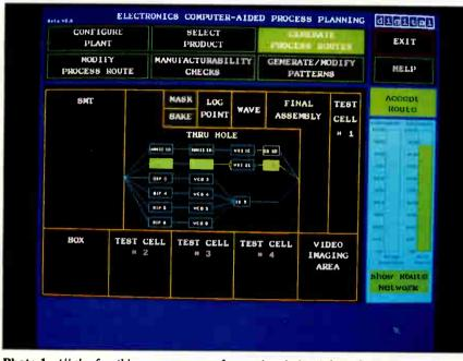
**Photo 1:** All the feasible process routes for a printed circuit board shown on a layout of the factory floor. The recommended route highlights the selected machines. Note in the "thermometers" on the right that the recommended route has an 85 percent automatic assembly with no setup required. (Photo courtesy of DEC)
