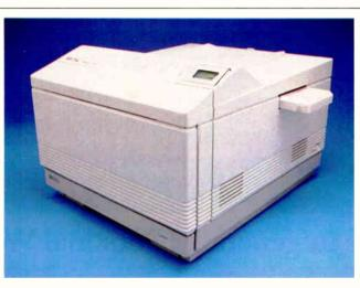
printer offers 512K bytes of memory and a solid 10-MHz 68000 processor. With memory upgrades and font cartridges, the IIP helped bring PostScript to general-business applications with a price tag that's under \$3000. Compared to its larger cousins, the IIP sacrificed some speed and duty volume, but it lost nothing in output quality and economy. For many users, this justified the cost of placing a laser printer on their desktops or beefing up their overall printing resources.
