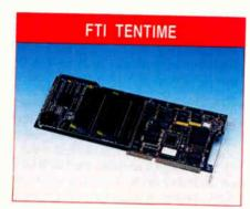
Like many other caching controllers, TenTime from FTI acts less like a controller and more like a dedicated coprocessor board. It has a 68070 CPU that executes a proprietary real-time, multithreaded operating system. The operating system supports error correction and intelligent cache management (the details of which the people at FTI were understandably reluctant to reveal).
