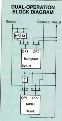
Figure 2a: The multiplier and adder can receive inputs from registers, their own outputs, or each other's outputs. They can be wired 62 different ways to create special-purpose instructions, such as "multiply-accumulate." set of possibilities. The adder, for example, can receive operands from floatingpoint registers, the special T (temporary) register, the multiplier, or itself.
