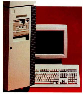
The CCS 486-25c EISA features a Mylex MAE486-25 motherboard with a Phoenix BIOS. Its 128K bytes of write-back cache provides zero-wait-state operation.
