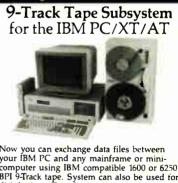
Now you can exchange data mes between your IBM PC and any mainframe or mini-computer using IBM compatible 1600 or 6250 BPI 9Track tape. System can also be used for disk backup. Transfer rate is up to 4 megabytes per minute on PCs and com-patibles. Subsystems include 7" or 10½" streaming tape drive tape coupler card and streaming tape drive, tape coupler card and DOS compatible software. For more information, call us today!
