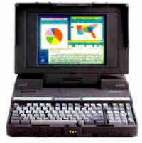
T5200C. 386 microprocessor, 200MB HDD, 2 to 14MB RAM, 2 IBM-compatible expansion slots (in addition to dedicated memory slots), VGA passive matrix color LCD display.
