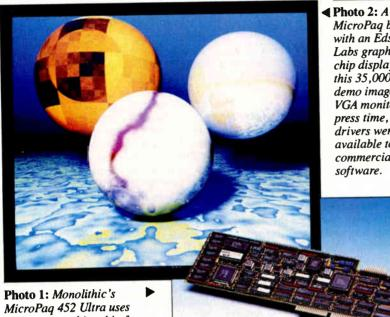
MicroPag board with an Edsun Labs graphics chip displayed this 35,000-color demo image on a VGA monitor. At drivers weren 't available to run commercial
