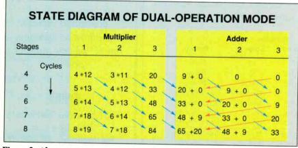
Figure 3: After seven cycles, partial sums begin to accumulate as the adder's results recirculate back through the adder.
