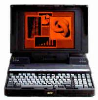
T5200. 386 microprocessor, 40, 100 or 200MB HDD, 2 to 14MB RAM, 2 IBM-compatible expansion slots (in addition to dedicated memory slots), VGA plasma display.
