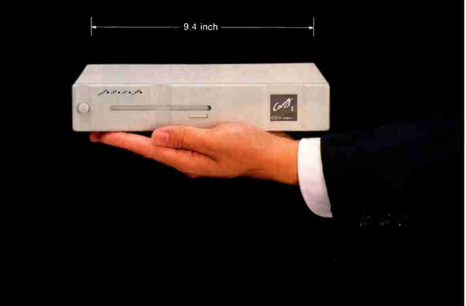
The Carry-I 9300 80386SX. 4M-byte RAM, 80M-byte Harddisk. One Expansion Slot, VGA...
