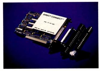
Adac's Direct Connect 5508HR data acquisition board.
