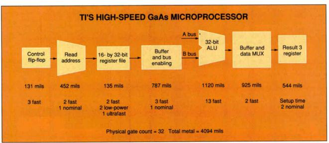
Figure 3: This critical path analysis shows the trade-offs made in TI's chip between speed and power requirements (which are directly proportional in GaAs technology). Propagation delay due to metal interconnects is significant, increasing the critical path delay by 25 percent. Note that the design concentrates 13 fast gates at the ALU, where a 1120-mil interconnect would otherwise slow processing significantly.
