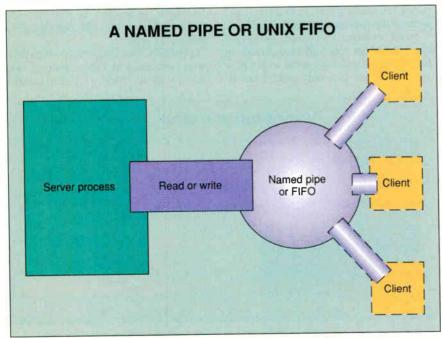
Figure 2: Named pipes do not require a parent-child relationship between the communicating processes. The client processes can come and go independently from the server.
