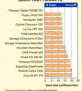
Figure A: Raw seek times measured by the BYTE Lab compare roughly with vendor-specified average seek times,
