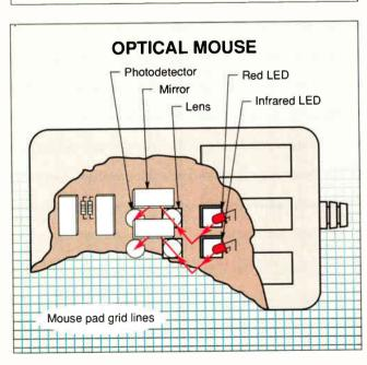
Figure 3: Red and infrared LEDs shine from an optical mouse onto a special pad. Reflected beams pass through lenses, then reflect onto photodetectors.
