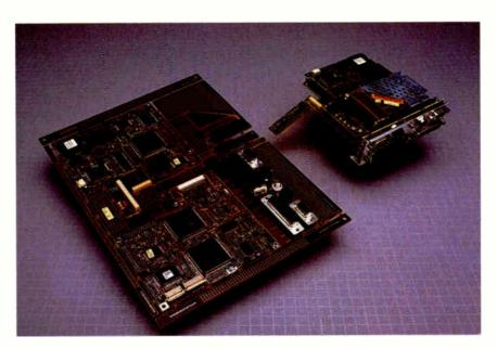
Photo 2: On the left is the LTE 386s/20 motherboard before it is punched out from its silicon casing. On the right is the motherboard as it is installed in the computer.
