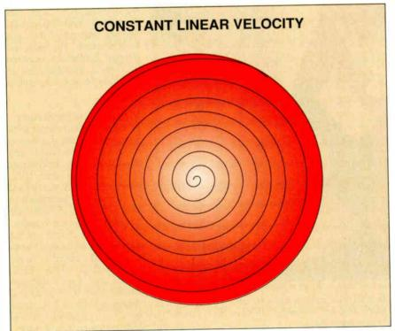
Figure 1: In constant linear velocity (CLV) recording, data is arranged in a single spiral track with a uniform density of bits. This lets you pack the most information possible onto the disk. The speed of the disk varies between the outer and inner edges—the closer the read head gets to the outer edge, the faster the disk spins. Data is located by its temporal position, measured in minutes and seconds. Each second consists of 2K bytes of data.
