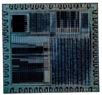
Photo 1: The FCI10. On the bottom left of the dye, the ALU path is set up so it will do 8-, 16-, or 32-bit operations. The large block at the lower right contains the hardware to implement the special instruction set that performs fuzzy-logic operations.
