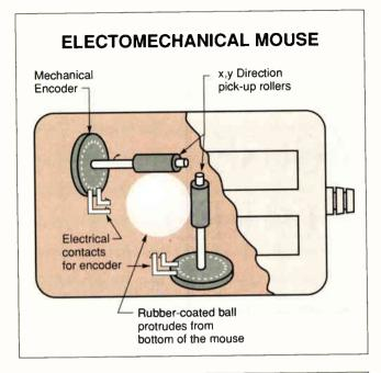
Figure 1: In an electromechanical mouse, a rubber ball drives the encoders, which make and break electrical contacts.
