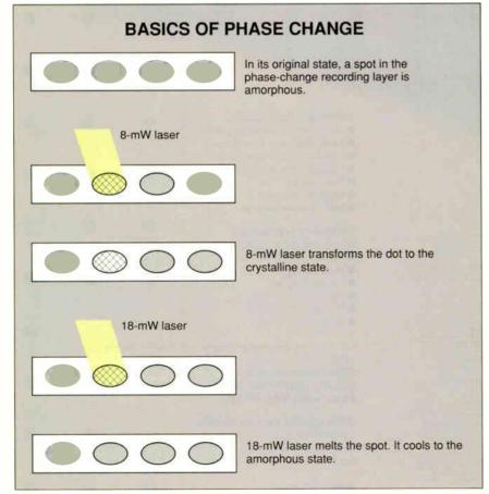
Figure 3: The remarkable property of phase-change media to change from amorphous to crystalline at one energy level and from crystalline to amorphous at a higher level enables the realization of direct optical overwrite.
