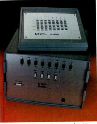
You can remotely control up to four VGA displays from eight systems with Network Technologies' matrix switch (bottom) and remote-control unit (top).
