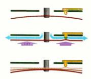
You don't want to entrust your data to anything you have to pamper. That's the beauty of Bernoulli. Its patented design spins a flexible disk at high speed, drawing it toward the head. Should your system encounter a bump, air impurity, or power-loss, the flexible disk simply falls away from the head. The result? Hard-disk performance without the risks.
