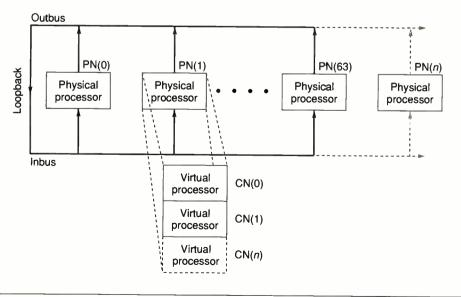
Figure 1: Adaptive Solutions' architecture can be extended in two directions. Each chip has 64 processor nodes, and additional chips can be added to provide arrays of hundreds of processors. Virtual processors, called connection nodes, are mapped to each physical processor, creating thousands of neural-network nodes. Loopback techniques and broadcast from any processor allow arbitrary interconnection of all nodes.
