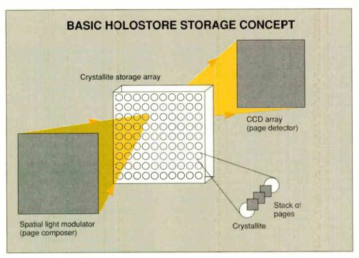
Figure 2: The holostore superimposes a pattern of light and dark spots based on the digital data onto the data portion of the laser beam. The data is stored as electronic-charge patterns. based on the interference between the data and reference beams, which modify the optical properties of the crystallite. The result is a 3-D holographic image of the bit pattern carried in the data beam.
