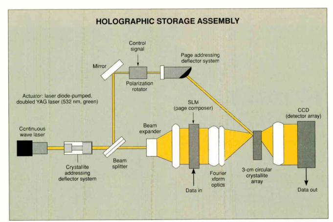
Figure 3: The laser source for the holostore prototype is a compact, doubled, diode-pumped YAG laser with 80-milliwatt output at 532 nanometers. The beam splitter splits the laser into separate data and reference beams and steers them onto the surface of a crystallite to store (or retrieve) a page of data.
