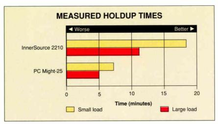
Figure 1: Holdup times for typical small and large loads, in minutes.
