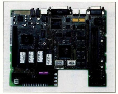
Photo 1: The Mac LC's logic board has a low component count due to the high level of logic integration. On the left edge is the 68020 Direct Slot; near the right edge are the SIMM sockets for RAM and the SIMM-mounted ROM.
