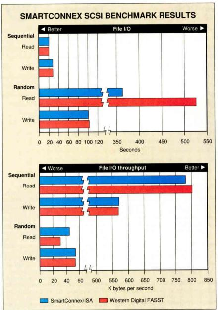
Although the SmartConnex/ISA can simplify upgrading to SCSI, its performance was only marginally better than that of the Western Digital controller that shipped with the test 300-MB SCSI hard disk drive.
