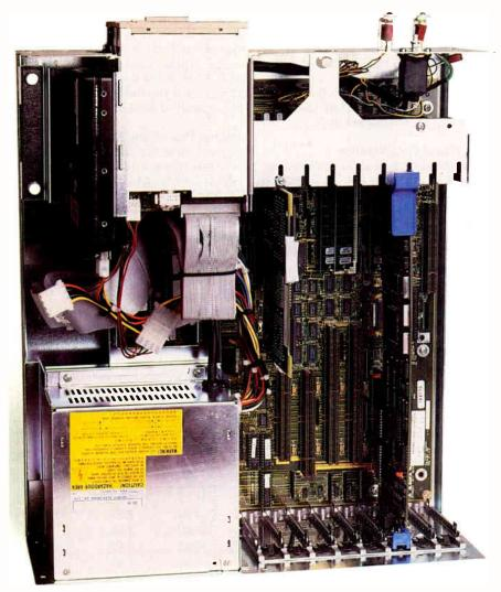
Photo 2: You can upgrade ALR's CPU module (the 486/25 with a Weitek socket is shown here) in about 5 minutes. You don't need to upgrade the software or firmware.
