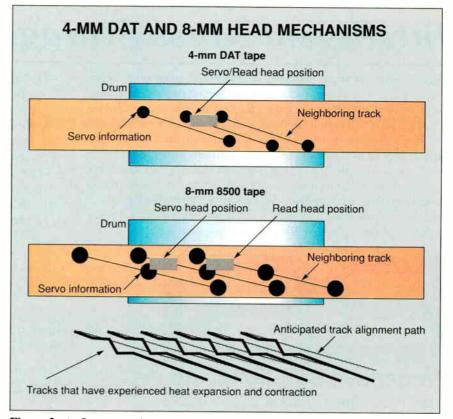
Figure 2: An 8-mm tape drive's separate servo and data heads can have trouble following distorted tracks. The 4-mm DAT drive's integrated servo and data heads track more faithfully.
