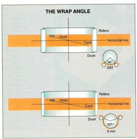
Figure 1: A DAT system's smaller wrap angle reduces friction during normal operation and prevents stretching of the tape during high-speed searches.
