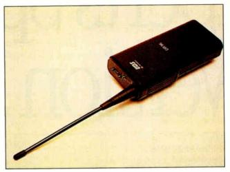
The DR 96 is a wireless, battery-powered modem for portable communications.
