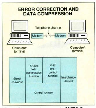
Figure 2: Many new modems now use the CCITT V.42 errorcorrection and V.42bis data-compression Recommendations. In the modem, these functions are located in the overall control processor and are applied to the signal between the computer and the signal converter (modulator/demodulator). Modems at both ends of the connection must have V.42 and V.42bis capability for these features to be used.
