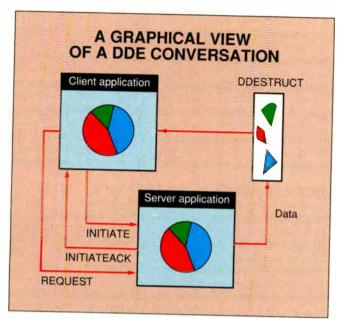
In a typical DDE conversation, the client initiates the conversation, and the server acknowledges. The client then requests data, which the server puts in shared memory.
