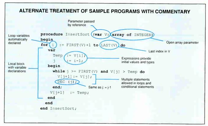
Figure 2: Although Modula-3 looks very much like Pascal and Modula-2, declarations can incorporate initial values, and data typing can be implicit.
