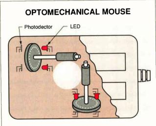
Figure 2: As with an electromechanical mouse, a rubber ball inside an optomechanical mouse drives the encoders. In this case, however, LEDs shine through holes in the encoders. The optical encoding scheme eliminates wear on the encoders.
