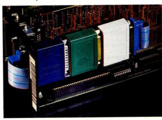
Software Security's adapter brackets hold a line of hardware security keys in place.
