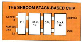
Figure 2: ShBoom has separate 32-bit internal buses for address and data. Both access the CPU, its two stacks, and the I/O processor. These buses are multiplexed into a single 32-bit external bus with DRAM and I/O control signals.
