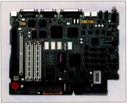
Photo 2: The Mac IIsi board combines on-board video and support for either a NuBus slot or a 68030 Direct Slot via a special adapter. This adapter plugs into the connector on the board's left edge. By the connector is one socket for SIMM-mounted ROM and four SIMM-mounted RAM sockets. At the center are crystal oscillators for the on-board video and bus clock. The sound I/O jacks are at the upper right.
