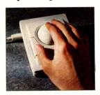
One button lets you pull down a menu or open a window. The other button can be set to "click-lock" for extended selections like automatic scrolling.
