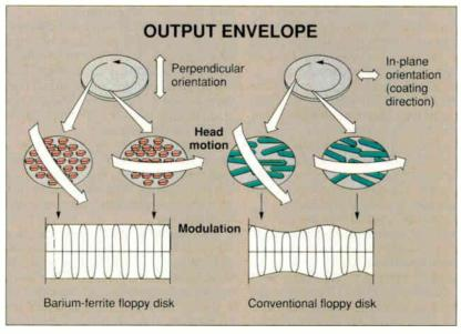
Figure C: Barium ferrite particles are flat platelets and provide a relatively flat data surface and a strong, continuous read signal (left). However, the media particles of conventional floppy disks exhibit different magnetization and shape characteristics and a fluctuating read signal (right).
