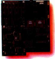
buffer card for ultra high-performance workstation graphics. For UNIX Workstations, Too. The 4860 board makes a great foundation for high-performance RISC workstations
