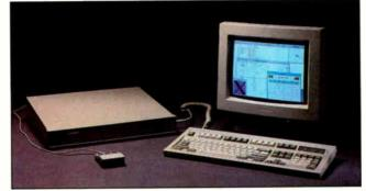
The Genisys 9000 supports local and network DOS processing, terminal access to multiple host databases, X Window System networking, and graphics.
