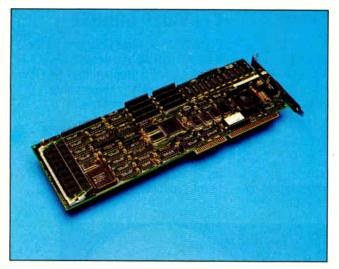
A 60-MHz TMS34010 graphics processor on the Hercules **Graphics** Station card accelerates TIGA-VGA throughput in resolutions of up to 1024 by 768 pixels by 8 bits. With the Art Dept. option, the card offers 24-bit color on standard VGA monitors.
