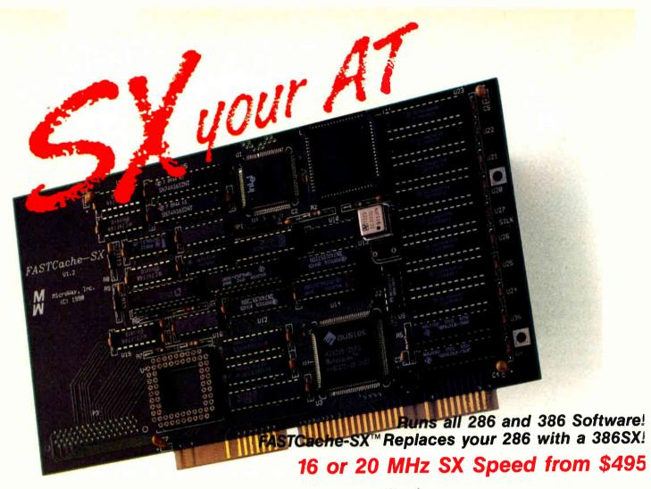
If you currently use an 80286 and are hamstrung by the 640K memory limit or need more speed, you owe it to yourself to try a Microway accelerator. The FASTCache-SX plugs into your 80286 socket replacing it with a 16 or 20 MHz 80386SX. It is fed by a large four-way cache similar to the one built into the 80486. This results in zero wait state performance using ordinary AT memory.
