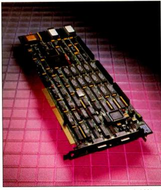
The DrawingCard MCA graphics board fits into a single 16-bit slot on your IBM PS/2 or compatible.
