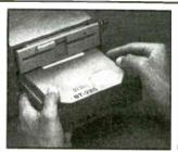
You install the 1.2 meg, 51%" floppy diak drive, learning disk drive operation and adjustment. Later, you improve your data storage capacity dramatically by installing this powerful 20 meg hard drive.
