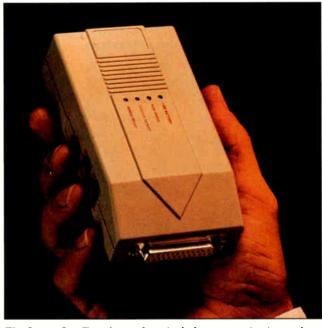
The Smart One Traveler package includes communication and fax software, a 9-V battery and external power supply, LED lights, a speaker, and a power-down feature.
