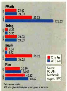
Using a 16Mkz 386: HIMEM driver and PC-DOS 3:3. Hard disk and RAM drift optimized between lests; compiled benchmark programs ren fram RAM drift. Each compiler was optimized for speed.
