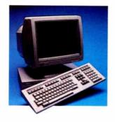
DEC introduces its first RISC-based workstation, the DECstation 3100.
