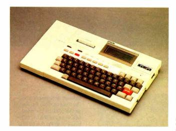
Epson America shows the HX-20, perhaps the first laptop computer; the machine weighs less than 3 pounds and uses a CMOS version of the 6801, 16K bytes of RAM, and a 20character by 4-line display.
