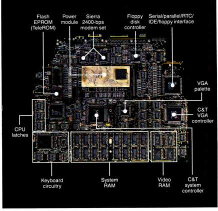
**Photo 2:** The VH-286 motherboard makes extensive use of surface-mount technology. It has a number of wire jumpers, which should not appear on the final production units.
