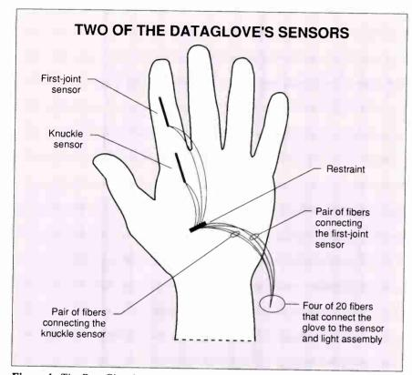
Figure 1: The DataGlove's sensors are glued to the glove, arranged directly over each joint. Loose fibers connect each sensor to a light source/receiver pair for measurement.
