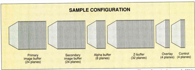
Figure 3: A frame buffer can have many bit planes and require a vast amount of memory. This configuration has a total of 96 bit planes. Assuming a screen resolution of 1280 by 1024 pixels, this represents 125,829,120 bits, or nearly 16 million bytes.
