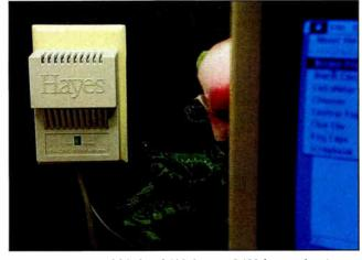
The Hayes Personal Modem 2400plus is a 2400-bps modem in an AC adapter.
