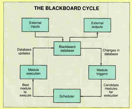
**Figure A:** A blackboard system lets multiple modules work on the same input. In an interactive-tablet system, the modules might consist of a neural network, lexical insertion, and a spacial parser.
