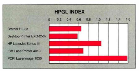
Figure 4: The HPGL Index. Three of the printers support the Hewlett-Packard Graphics Language internally. A fourth, the Desktop Printer EXO-2507, packages software emulation. The LaserJet Series III, driven by HP's latest incarnation of its Printer Control Language (PCL 5), incorporates HPGL commands into its command set. The index is based on the Series III results. Long bars indicate superior performance. The PCPI LaserImage 1030 produced the sharpest plots in record time.
