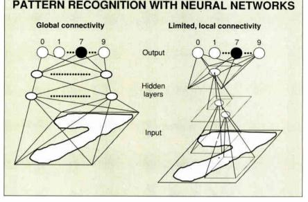
Figure 1: Back-propagation techniques enable a neural network that starts out with randomly valued connections to learn to correctly recognize input patterns. Network architectures with limited connectivity represent one way to make these recognition systems compact enough to fit on small machines.
