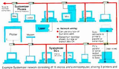
Example Systemizer network consisting of 11 micros and a minicomputer, sharing 3 printers and a modem via a mixture of Systemizer Pluses and Systemizer SCs. Note: though not shown here, some of the computers could also be connected to a traditional LAN or WAN.
