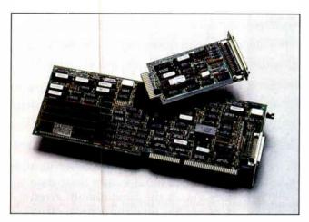
The StellarPS full-size controller board holds Intel's new i960 RISC chip. The smaller video adapter board plugs into a LaserJet Series Il printer.
