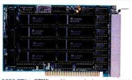
The PCSS-8TX is GTEK's workhorse multi-channel serial I/O card with compact RJ-11 telco jacks. The PCSS-8TX provides 8 standard uarts arranged as either COM1/COM2, or memory mapped. Also available is the PCSS-8X with DB-25 connectors. For SCO™ XENIX® order the PCSS-8TH.
