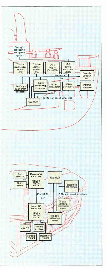
Figure 2: Two different methods of telemetry connecting the computer suite on the mother ship through the Medea camera ship to Jason. On the left, standard serial lines connect Jason's computers, while on the right, an updated scheme uses a LAN to connect system components. Both options use the fiber-optic cable, but the network telemetry shown at right addresses the vehicle as an actual node on a 10-Mbps LAN. This network can then be easily connected to other networks via a satellite link.
