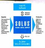
36 digital/analog input/output channels are compatible with standard sensors and cutput devices. SOLUS can be located on site, or remotely via modem.
