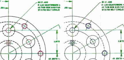
Two sample Vellum CAD drawings, one from the HP 7475A pen plotter (left) and one from the Da Vinci RasterPro 720 using 7475A emulation. While the HP pen plotter boasts more vibrant colors, the RasterPro comes very close to matching its output. It even drew smaller figures with greater clarity than the HP plotter.
