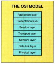
Figure 1: The OSI Model consists of seven protocol layers that allow dissimilar computers and applications to communicate and share data. Wireless LANs concern themselves with the Physical and Data-link layers of the model, which describe the physical nature of the connection between two machines and an error-free method of data transmission over that connection.
