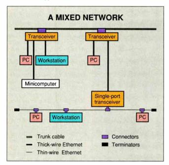
Figure 1: Through the use of a thick-wire/thin-wire single-port transceiver, machines using both thin-wire and thick-wire Ethernet can all communicate.
