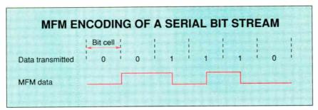
Figure 3: MFM encoding (like RLL encoding) merges data and clock information into a single, combined signal.
