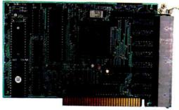
The PCSS-8I is GTEK's most popular intelligent serial I/O card with compact RJ-11 telco jacks. It provides 8 serial channels for PC/XT/AT/PS2-286 and is DOS Compatible. The PCSS-8I has 32K of *Dynamemory*, user upgradeable to 128K bytes. Driver available for SCO™ XENIX®
