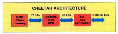
Figure 1: The Cheetah 433 AT Gold architecture allows 32-bit writes to the I/O controller. The controller then sends the message over the slower AT bus, freeing CPU cycles for memory accesses.
