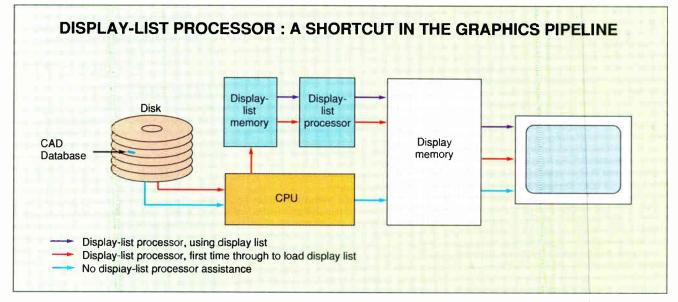
**Figure 1:** A display list is a special kind of cache that stores endpoints to define the line segments of a CAD image. Once you've built a display list, there's no need to revisit the database or repeat vector calculations. This makes most pans, zooms, and redraws almost instantaneous.
