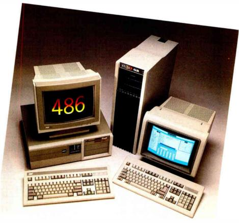
**Photo 1:** The AST Premium 486/33 (left) is a desktop design with an ISA bus, while the ALR PowerVEISA 486/33 sports a tower design with an EISA bus. AST offers EISA versions in both desktop and tower form.
