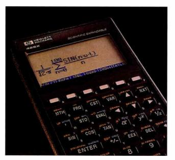
calculator to either Macintosh or DOS systems. In fact, the kit lets you control the calculator from the host computer, allowing you to use the calculator as an equation-solving peripheral. The calculator also has a twoway infrared interface for use with HP's infrared printer or for exchanging programs or data with another 48SX.
