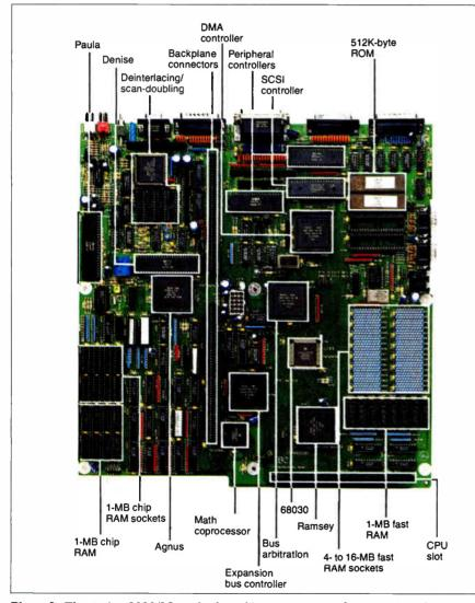
**Photo 2:** The Amiga 3000/25 motherboard integrates many functions into discrete chips. The expansion backplane connects to the two 100-pin sockets at left-center. Expansion boards thus lay parallel to the motherboard. Note the 200-pin CPU slot at right-front. (Food for thought: The 68040 comes in a 179-pin package.)
