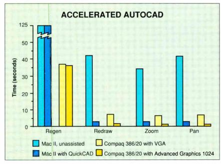
**Figure 2:** BYTE's AutoCAD benchmark tells the story: When both machines are unassisted, the Compaq 386 wallops a Mac II. But the Macintosh/QuickCAD duo stands shoulder to shoulder with a Compaq 386/34010 combo in those operations that can benefit from a display-list processor.
