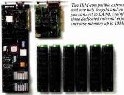
Two IBM-computible expansion slots (one full-length and one half-length) and an internal modem slot let you connect to LANs, mainframes and more. Plus, three dedicated internal expansion slots let you increase memory up to 13MB.
