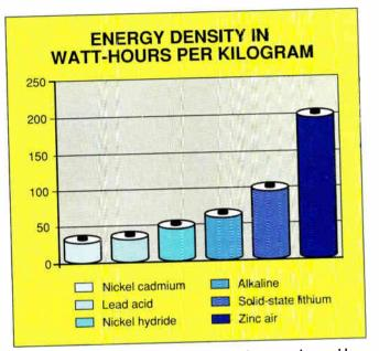
**Figure 2:** As this graph of power output shows, rechargeable nickel-cadmium batteries (currently favored for portables) and good old alkaline batteries may face stiff competition from zinc-air, nickel-hydride, and solid-state lithium batteries, which offer combinations of rechargeability, higher power, and longer operating life.
