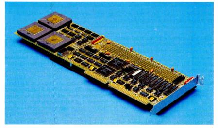
The Opus 88000 coprocessor card. The three large, brass-centered chips are the 88100 CPU and the dual 88200 cache/memory management units.
