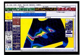
Lap CADII, analyzing the stress contours of an automotive suspension part.
