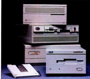
The LaserVault 650 is a rewritable optical drive with multiplatform SCSI drivers.
