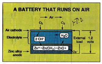
**Figure 1:** At one end, the Aerobic Power battery has a fairly typical zinc alloy anode. The cathode, however, features an air-breathing carbon membrane that extracts oxygen from the atmosphere. Oxygen and water are broken down into negatively charged hydroxide ions (OH<sup>-</sup>), which bond with positively charged zinc atoms, releasing water and electricity.
