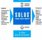
36 digital/analog input/output channels are compatible with standard sensors and output devices. SOLUS can be located on site, or remotely via modem.
