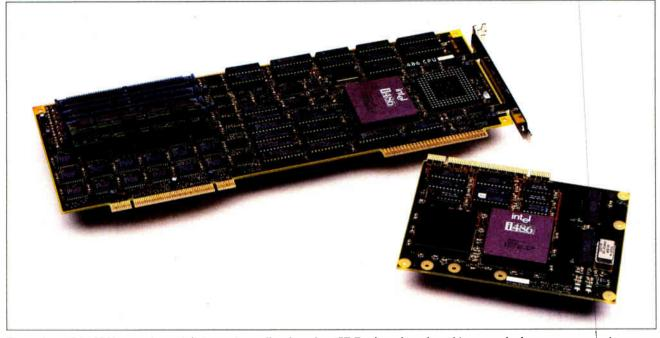
**Photo 2:** ALR's CPU upgrade module is much smaller than the AST Fastboard card, and it uses only the separate proprietary slot on the ALR motherboard. AST's card uses one of the standard 16-bit slots, as well as a proprietary 32-bit slot. Both designs make for simple upgrades.
