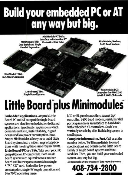
MiniModule Expansion. Extend your Little Board based embedded system using Ampro MiniModules. These compact 3.5" X 3.8" boards provide CGA or EGA video interfaces,
