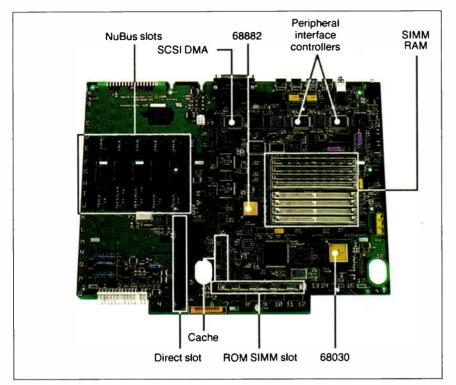
The Mac IIfx's logic board represents a new design. Although it has new functions such as cache memory and peripheral controllers, the IIfx board has the same chip count as the IIci logic board. Note the empty real estate on the board, suggesting that a compact model with fewer slots could also be produced.
