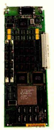
The 8/24 GC graphics accelerator board. Note the AMD29000 RISC processor, which operates at 30 MHz. The board comes standard with 2 MB of video RAM and includes a 64K-byte static RAM instruction cache.
