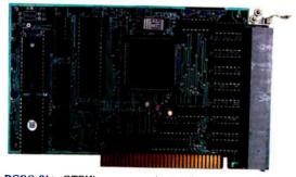
The PCSS-81 is GTEK's most popular intelligent serial I/O card with compact RJ-11 telco jacks. It provides 8 serial channels for PC/XT/AT/PS2-286 and is DOS Compatible. The PCSS-81 has 32K of **Dynamemory**, user upgradeable to 128K bytes. Driver available for SCO<sup>C™</sup> XENIX<sup>®</sup>.
