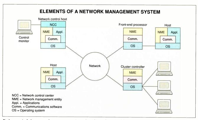
Each system includes a network management entity package that performs local functions. It can communicate with a network control center that has the same software as other nodes, plus network control software that provides a user interface for managing the entire network.
