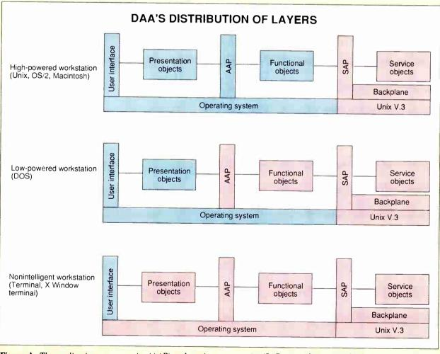
Figure A: The applications-access point (AAP) and service-access point (SAP) are industry-standard remote procedure calls that allow you to configure DAA for different workstations. Notice how the distribution of layers depends on the sophistication of the workstation used. (The red shows the portion residing on the server; the blue shows that on the clients.)
