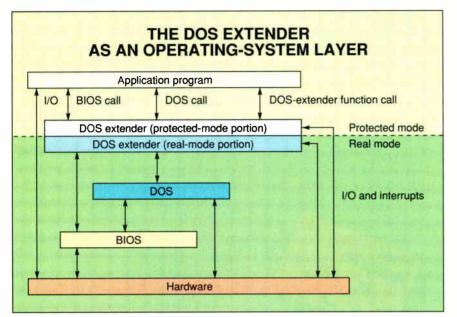
A DOS extender accepts DOS and BIOS calls from a protected-mode application, processes the parameters, and reissues the request in real mode. It also fields interrupts in protected mode (and some in real mode as well), performing mode switches and reissuing interrupt requests as necessary. A DOS-extender application can also have a portion that runs in real mode (not shown), usually for the purpose of handling interrupts without a mode switch.
