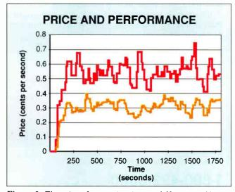
**Figure 3:** The price of computing time on different machines is different if the machines have different capabilities. The dark line shows the price of time (established by auction) on the faster and consequentially more valuable Sun-4/260. The gray line is the price of computation on a Sun-4/100.
