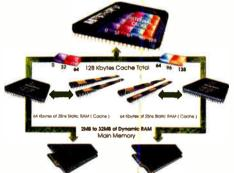
PowerCache 4 is the first PC to fully utilize 128-bit burst mode and a "read and writeback" 128KB cache design, providing better than zero wait state performance as compared to the i386.
