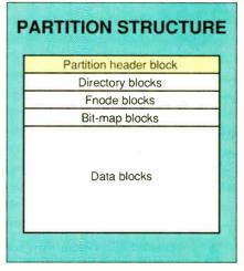
**Figure 1:** The partition header block is always the first 1024 bytes of the partition and carries parameters that define the other regions' sizes and locations.
