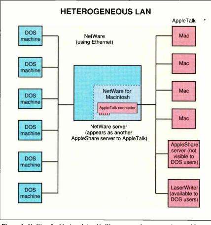
**Figure 1:** NetWare for Macintosh is a NetWare process that communicates with AppleTalk via an AppleTalk connector. The gateway lets DOS users access AppleTalk printers and AppleTalk users access the NetWare server.
