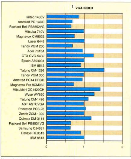
**Figure 3:** The VGA index is a weighted geometric mean of the other indexes, emphasizing line width and misconvergence. Monitors are listed according to price, with inexpensive models at the top. Long bars reveal outstanding performers, so look for long bars at the top of the graph. For example, while the Laser 6448 and the Zenith ZCM-1390 have similar indexes, the Laser delivers a higher price/performance mix.
