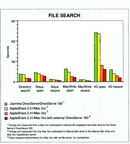
Figure 3: The benchmarks use MPW's Whereis command to search for a nonexistent file and report the time necessary to zip through the benchmark folder. In addition, I timed file opening and resaving using a 30K-byte Nisus file, a 70K-byte MacWrite II file, and a 2.5-megabyte 4th Dimension file. Times are the average of 10 repetitions in seconds.
