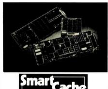
Not just a memory cache, but an intelligent controller card with advanced caching features such as: automatic disk read-ahead and elevator sorting during cache writeback.
