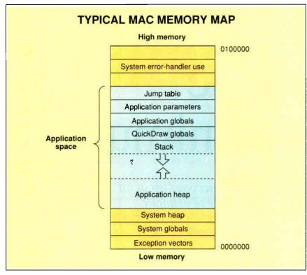
**Figure 1:** A generic memory map for Macintosh computers. Your application runs in the application space. The Mac Plus and SE screens and sound buffers are located in high memory. The QuickDraw globals and jump table are used to manage the operation of the application and maintain its graphical user interface.
