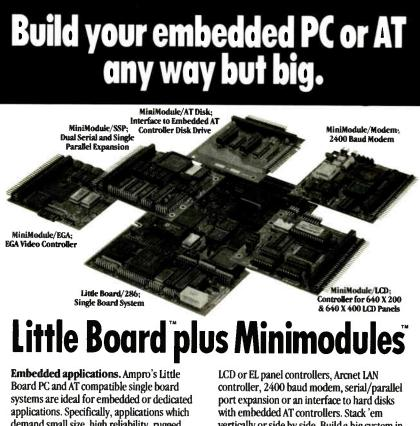
demand small size, high reliability, rugged design and low power consumption. Now, Ampro MiniModules allow you to build Little Board systems into a wider range of applications while meeting these same requirements. Little Board/PC or /286. Take your pick. PC compatible or AT compatible. Both single board systems are equivalent to a motherboard and four expansion cards in a single 5.75" X 8" card. Both offer low power consumption, single 5V supply operation and 0 to 70°C operating range.
