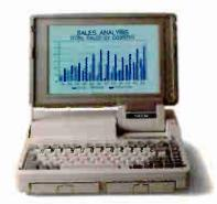
T1600: Battery-powered 80C286/12MIII, 20MB and 40MB hard disk models, 1.44MB 3½ diskette drive, 1MB RAM expandable to 5MB, detachable backtit EGA-compatible LCD, removable rechargeable battery pack, coprocessor socket, 7 standard interfaces, 2 Toshiba slots for general purpose options.
