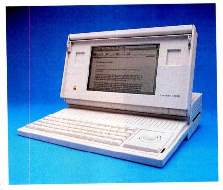
blurry by comparison. But the lack of a backlight on the Mac Portable means that you can't use the machine in a darkened airplane cabin or in other areas that are poorly lit.
