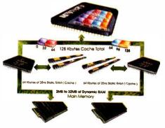
PowerCache 4 is the first PC to fully utilize 128-bit burst mode and a "read and write-back" 128KB cache design, providing better than zero wait state performance as compared to the i386.
