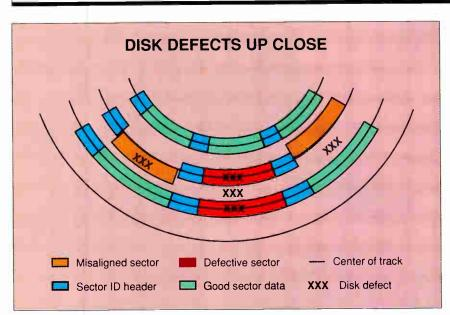
A disk can have defects caused by a misaligned data sector, a faulty data sector, or faulty media, as illustrated here.
