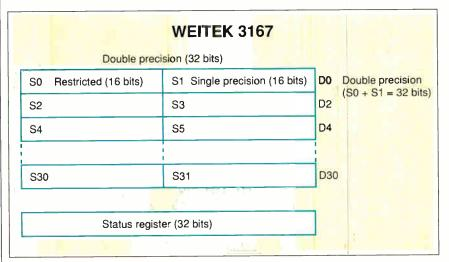
Figure 4: Although the registers are only 32 bits wide, they can be paired for 64-bit operations. There is no provision for double precision extended. The Weitek 3167 uses the address bus for instructions in order to increase throughput.
