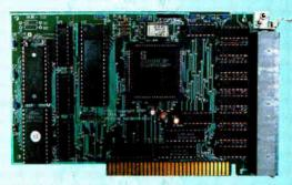
The PCSS-8I is GTEK's most popular intelligent serial I/O card. It provides 8 channels for PC/XT/AT/PS2-286 and is DOS compatible. The PCSS-8I has 32K of Dynamemory, user upgradeable to 128K bytes. Dynamemory dynamically allocates buffer ram as need.
