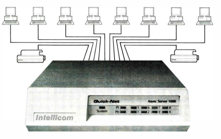
The Quick-Net Async Server 1000 offers the multi-PC office a ow cost alternative to expensive and complicated LANs. The Server 1000 features 8 serial ports and 2 parallel ports. With his Server up to 9 users can share a printer. Multiple printers can also be shared in a variety of ways including general or selected user access.
