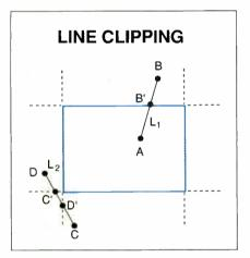
Figure 4: The clipping of line  $L_1$  is successful, since the software can project point B to point B'. The clipping of line  $L_2$  fails—projecting C to C' and D to D' produces a segment that is still outside the window.
