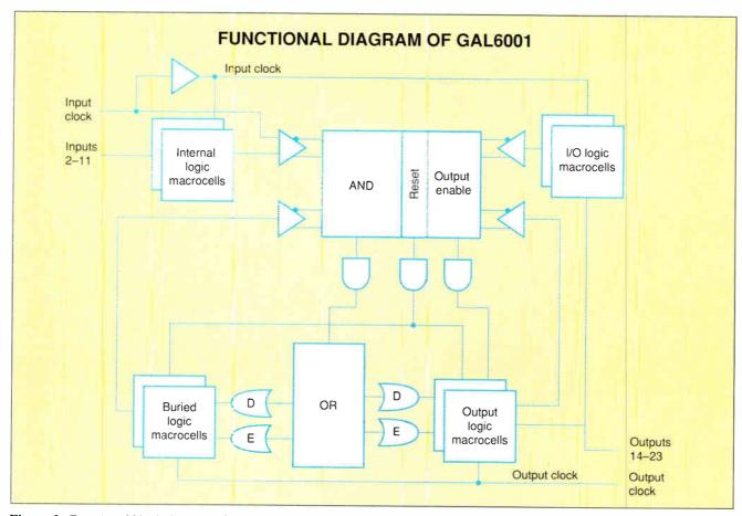
Figure 3: Functional block diagram of the GAL6001. This device offers such complexity that it's easy to run out of pins.
