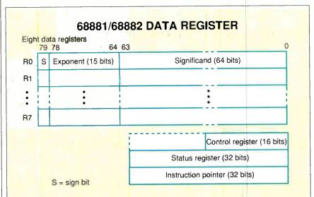
Figure 3: This also has 80-bit-wide registers. The 68000 can manage more than one FPU at a time. The Motorola FPU registers cannot be used as a stack.
