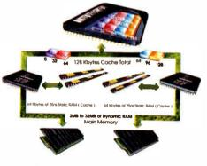
PowerCache 4 is the first PC to fully utilize 128-bit burst mode and a "read and write-back" 128KB cache design, providing better than zero wait state performance as compared to the i386.
