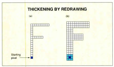
Figure 9: Another route to thicker characters. (a) A 1-pixel-thick letter F. (b) A thick letter F is created by redrawing the 1-pixel-thick character while stepping the starting pixel around the perimeter of a square.
