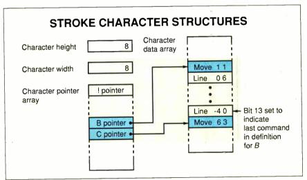
Figure 6: Data structures for defining stroke characters. Each printable character in the character set is associated with a pointer in the character pointer array. Each pointer indicates an offset into the data array where the commands defining the character begin.
