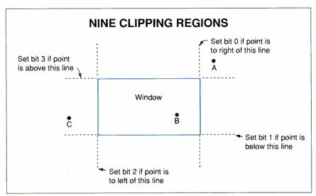
Figure 3: Matching point coordinates with the window boundaries, the graphics software determines where a point lies in relation to the clipping window. So point A would return a clipping code of  $1001_2$ ; point B,  $0000_2$ ; and point C,  $0100_2$ .
