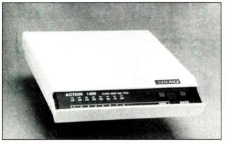
When your leased line is interrupted, the Action 1496 modem will automatically use its V.32 dial-up protocols and connect you at 9600 bps.
