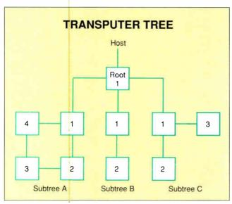
A tree of transputers is divided into as many as three subtrees attached to the three nonhost links of the root transputer. The subtrees can be any valid transputer configuration.
