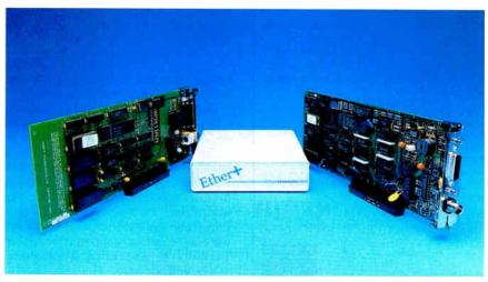
Left to right: Asante Technologies' MacCon II/E, Compatible Systems' Ether+, and Apple's EtherTalk NB.
