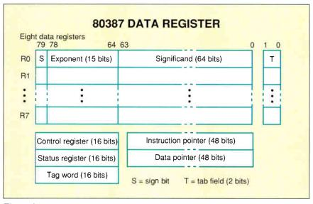
Figure 2: Each register is 80 bits wide. Only one 80387 can be used on the system at a time. The registers can be used as a stack.
