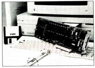
The MacAdios II Ir lets the Macintosh II run laboratorymeasurement and process-monitoring applications.
