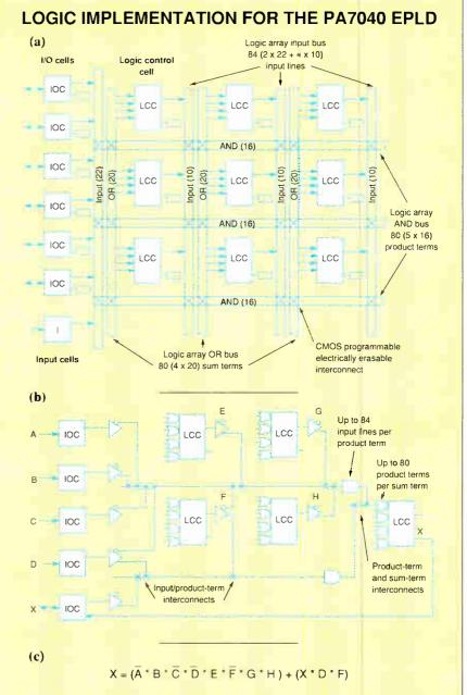
Figure 4: (a) A section of the distributed logic array matrix for the PA7040 EPLD; (b) a sample logic diagram; and (c) the Boolean expression that produced it.
