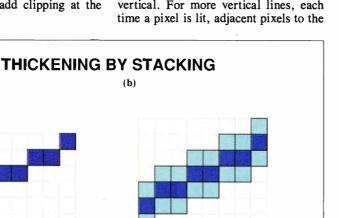
Figure 8: (a) The software draws a 1-pixel-thick line. In order to draw the thick line (b), the software treats each pixel of the line as the midpoint of a vertical line segment. This thick line is composed of vertical segments because it is more horizontal. Thick lines that are more vertical are composed of horizontal segments.
