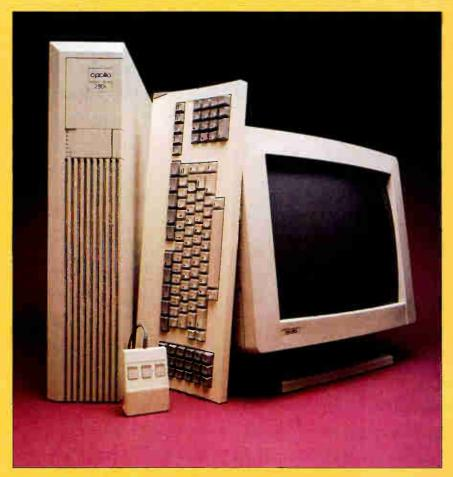
The Apollo 2500 provides workstation performance for less than \$4000. Note the unusual keyboard layout designed for use with Apollo's proprietary Domain/OS.
