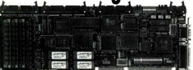
One philosophy. Two systems. Ampro's new Slot Board/286, like the Little Board/286, is a complete ATcompatible single board system. Each is equivalent to an AT motherboard and four expansion cards. Now, you can choose between stackable systems with the Little Board/ 286 or passive backplane systems with the Slot Board/286.
