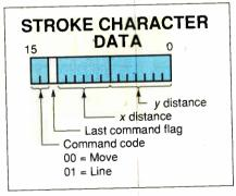
Figure 7: The format of an entry in the character data array. The last command flag is set to 1 to mark the end of a character's definitions. Both the x distance and the y distance fields are stored in two's complement form to allow drawing in negative as well as positive directions.
