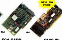
640 X 350 HIGH RESOLUTION • DISPLAYS 16 COLORS AT A TIME . COMPATIBLE WITH HERCULES, CGA AND IBM MONOCHROME . SOFTWARE DRIVERS FOR WINDOWS, LOTUS, CAD, AND MORE + 256K VIDEO RAM MCT-EGA
