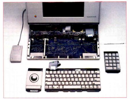
Photo 1: The keyboard and the trackball can be removed and swapped to accommodate left-handed users. Mouse users can replace the trackball with a keypad.
