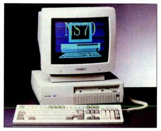
Normerel's 25-MHz NS70-25 has an MCA bus.
