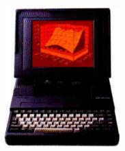
T3100e: 12MHz 80286, internal IBM slot, 20MB hard disk, gas plasma display, IMB RAM expands to 5MB, 1.44MB 3½" diskette drive.
