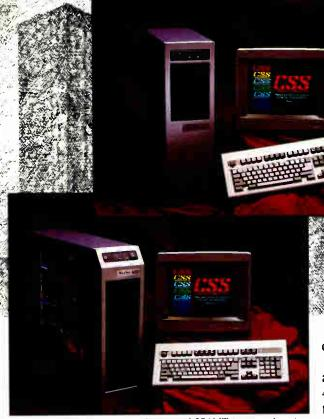
The MaxSys 386T (lower photo) and 386MT (upper photo) feature 12 slots to provide the systems with expandability.
