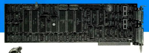
And think about OST, the European leader in the field of private X.25 networks! Our PC XNET card, an option/adapter card for personal computers, provides two channels, each supporting 128 virtual circuits and speeds to 64 kbps. The PC XNET card provides a level of performance never before reached in a personal computer.
