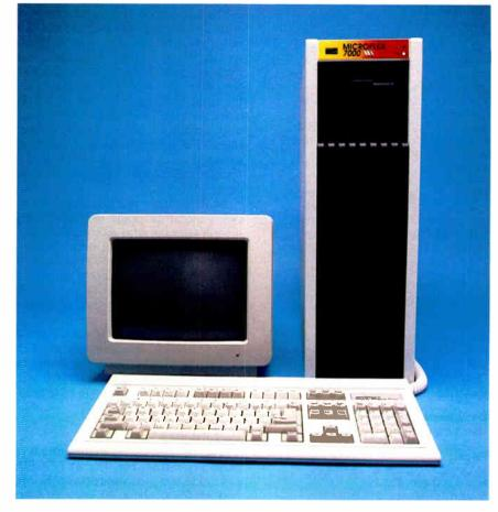
hard disk drive) costs \$8499, while the Model 300-A31 (with a 310-megabyte hard disk drive) runs \$12,397. Standard features include 2 megabytes of DRAM, a math coprocessor socket, SuperVGA circuitry, a 1.44-megabyte 3½-inch floppy disk drive, and an ESDI controller. Software includes an ALR Reference Diskette that lets you configure MCA peripherals; Multisoft's Super PC-Kwik disk cache; and Quarterdeck's DESQview and Expanded Memory Manager (QEMM-386).
