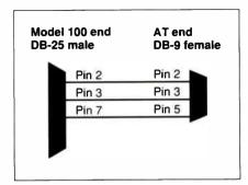
Figure 2: Diagram for a PC AT-to-Model 100 cable.
