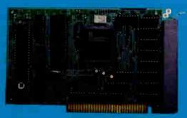
The PCSS is GTEK's most popular intelligent serial I/O card. It provides 8 channels for PC/XT/AT/PS2-286 and is DOS Compatible. The PCSS is has 32K of December, user upgradeable to 128K bytes.
