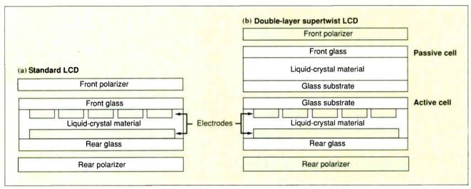
Figure 1: The major difference between the standard LCD (a) and the double-layer supertwist (DST) display (b) is the addition of a passive liquid-crystal layer in front of the active LCD layer. The additional layer reduces color distortion.
