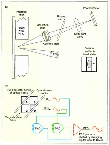
Figure 3: (a) The Floptical disk technology increases data density by using an optical track to generate precise tracking of the read/write head. (b) Alignment of the head to optical servo tracks is accomplished with a Phase Error Signal shift technique using multiple digital analog converters.
