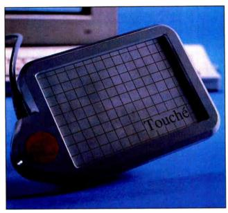
Touché, a touch tablet with a clear glass surface, provides absolute cursor control and mouse emulation.
