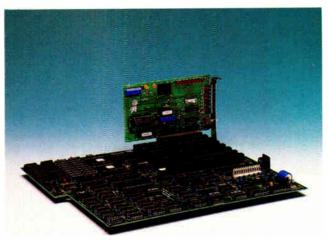
ward Software's aptly A named POSTcard is an add-in card that monitors your IBM PC during the POST (power-on self test) sequence that's run from the ROM BIOS every time you turn on your system. POSTcard has both a dual-digit LED display and a setup of 10 individual LEDs that tell you (in hexadecimal and binary, respectively) what tests are being performed. If your system locks up, it tells you exactly where the problem lies
