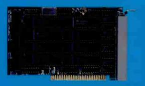
The PCS-IIX is GTEK's workhorse multichannel serial I/O card with compact RJ-11 telco jacks. The PCS-IIX provides 8 standard uarts arranged as either COM1/COM2, or memory mapped.
