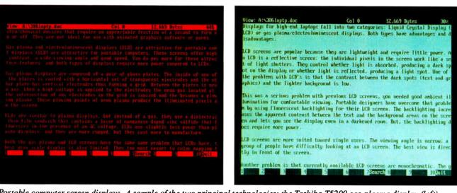
Portable computer screen displays. A sample of the two principal technologies: the Toshiba T5200 gas-plasma display (left) and the Zenith TurbosPort backlit LCD (right).
