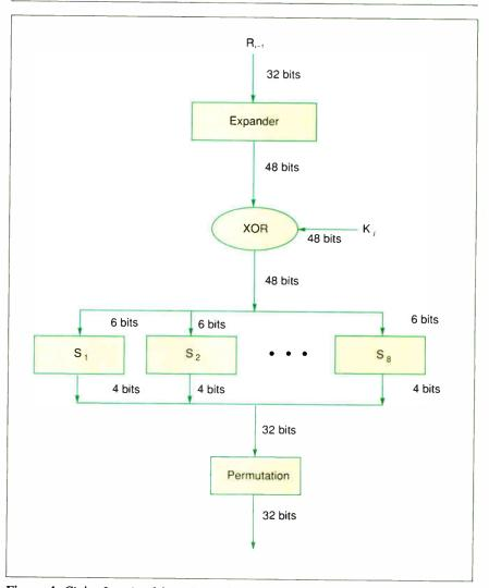
**Figure 4:** Cipherfunction f from figure 3. Its output comes from the old R part  $(R_{i-1})$  and the current key  $(K_i)$ . The inputs use eight S boxes to perform substitution and then permute their combined output to give the function's output.
