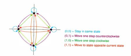
**Figure 2:** Four-state differential phase-shift keying. This phase-amplitude diagram shows a set of states and transitions for a four-state DPSK modulation scheme.
