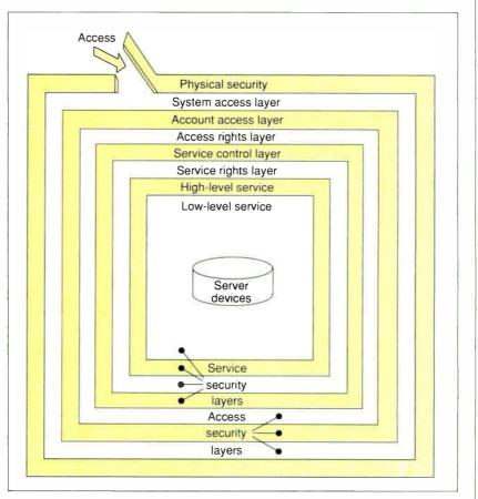
**Figure A:** Like an onion, good security is composed of layers wrapped on layers. In the file-server model, access to the actual device must go through three layers of access security and four layers of service security.
