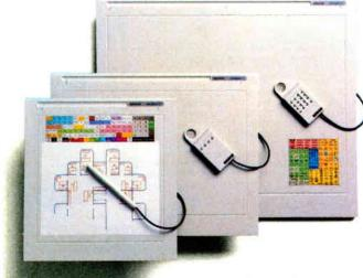
**1.** <u>Flexibility</u>. Quick menu picking. Also high resolution tracing and drawing. And selective resolutions of up to 1,016 lines per inch.
