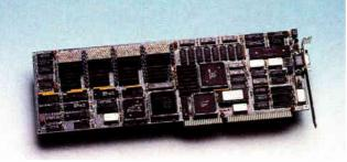
coprocessor card for CAD applications. The card, compatible with the MultiSync XL, packs 2 megabytes of video memory and displays 256 colors at 1024- by 768-pixel resolution. The Verticom HX-256/AT sells for \$3495. The card was not available for this evaluation.
