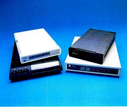
**Top of the Line:** (Clockwise from upper left): Fastcomm FDX 2448, Hayes V-series Smartmodem 2400 V.42, Telcor 2496MA, and E-Tech Bullet E2400M.
