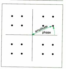
Figure 3: A Quadrature Amplitude Modulation constellation. Each point in the graph of a 16-point constellation represents a phase-amplitude state that the encoding scheme uses. CCITT V.22 bis uses a 16-point constellation.
