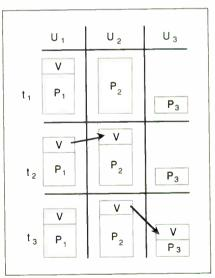
Figure 1: A picture through time of a virus infecting a system. A virus, V, infects user  $U_1$ 's program  $P_1$  at time  $t_1$ . At  $t_2$ ,  $U_1$  shares information with  $U_2$  and infects  $P_2$ . When  $U_2$  shares data with  $U_3$  at  $t_3$ ,  $P_3$  becomes contaminated. (Figure courtesy of Fred Cohen)
