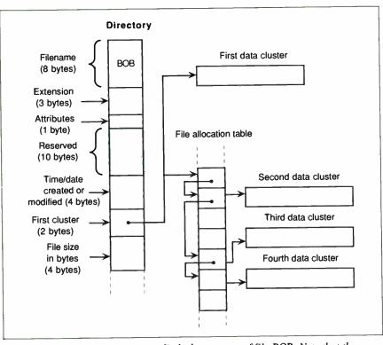
**Figure 1:** How an MS-DOS system finds the contents of file **BOB**. Note that the format of an MS-DOS directory entry is defined here.
