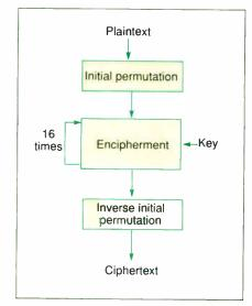
**Figure 2:** The DES encryption process. Every bit in the output is a complex function of every bit in the input block and every bit in the key.
