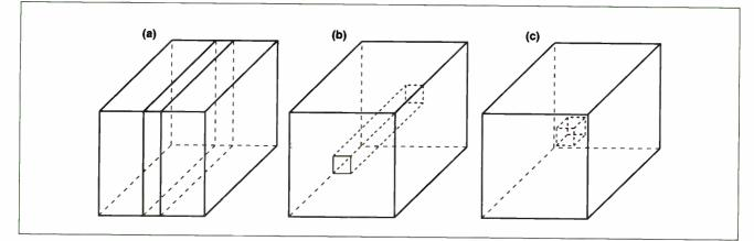
Figure 4: (a) Restriction by one dimension results in a quantum well; (b) restriction by two dimensions produces a wire; (c) restriction by three dimensions produces a dot.
