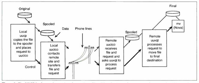
Figure 2: The UUCP background operations for copying a file. Although it is simple to generate the request for a file transfer, the actual operations of the UUCP daemons are more complex.
