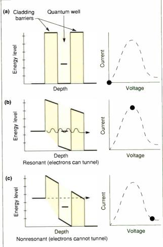
Figure 2: The different states of a resonant tunneling diode: energy level versus depth (left) and the corresponding voltage versus current (right). (a) When the energy level of the source contact is below the quantum state within the well, there is no tunneling. (b) When the source contact level is raised to match that within the well, tunneling occurs. (c) If the source contact level is raised even further, tunneling ceases since the level inside the well no longer matches that of the source.
