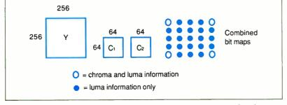
Figure A: Chrominance subsampling takes advantage of the fact that the eye has less spatial sensitivity to color than to brightness. Three bit planes, two of them at one-quarter resolution, are used to reproduce the image by interpolating colors between the points.
