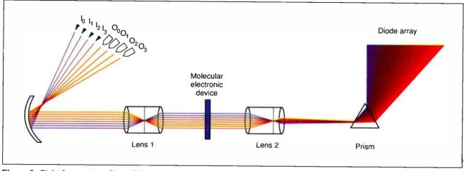
**Figure 2:** Eight frequencies of laser light (representing the four input and four output channels) are passed through the molecular electronic device, and the emerging light is read via the diode array (DA). Components in the MED can block the output frequencies of light or let them pass through. (Source: Center for Molecular Electronics, Syracuse University, Syracuse, NY)
