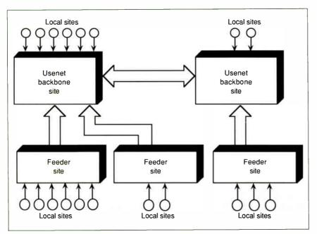
Figure 1: The relationship between the local site and the backbone site. Mailrouting functions exist between backbone-site machines. By consulting a map of all the intermediate sites and most of the leaf sites, UUCP can figure out a path for your message.
