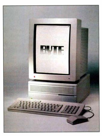
What is interesting about the Mac IIcx is its physical design and modular construction, which remind me of the IBM PS/2 series. The cover, power supply, and drive housings all have snap fittings made of high-impact plastic. This allows you to disassemble the entire machine in a few minutes.
