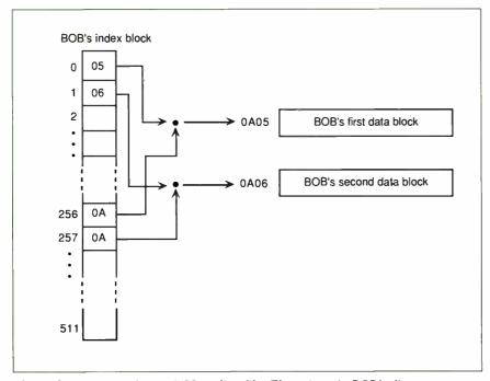
**Figure 3:** Structure of a ProDOS sapling file. The pointer in BOB's directory entry now leads to an index block. Notice that the word-wide block number of BOB's data blocks is formed by concatenating low and high bytes from opposite halves of the index block.
