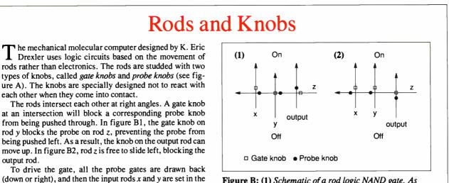
Figure B: (1) Schematic of a rod logic NAND gate. As long as the gate knob on either the x or y input blocks the intersection, the output rod is free to slide. (2) If x and y are both on, rod z is free to slide, blocking the output rod.
