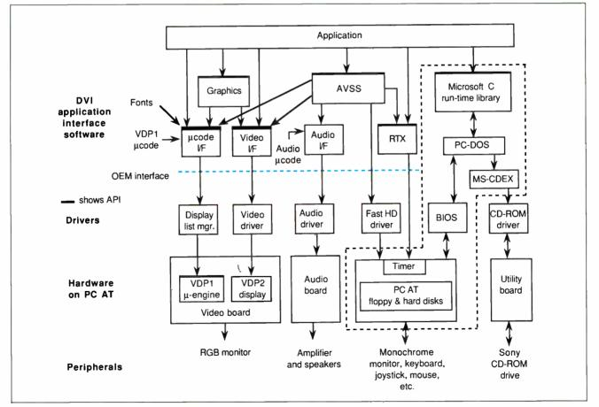
Figure 2: The digital-video-interactive run-time software is layered and modular. The low-level device drivers are implemented as TSR programs; the higher-level software is packaged as run-time libraries for the C language. There are facilities to directly execute custom microcode on VDP1.
