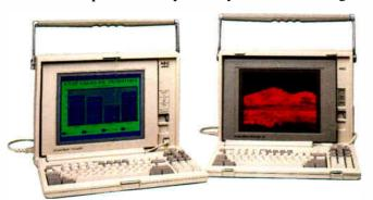
PowerMate Portable Intel<sup>\*</sup> 80286 microprocessor 10/8 M Hz speed memory to 4.6 M B EGA resolution on a back lit LCD display
