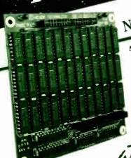
4 MB Memory Module for COMPAQ DESKPRO 386/20, 386/20e, and 386/25 Computers Now with NO FAITH THE COMMISSION OF THE COMM 4 MB Memory Module for CUMPAU DESKPRU 386/20, 386/20e, and 386/25 Computers. Now with NO-FAULT software at no extra cost! Adds up to 10MB of nign-speed memory.
