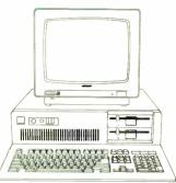
• Intel 8088-1Switchable from 4.77 to 10MHZ • 512K RAM Expandable to 640K • Dual Floppy Controller • 150 Watt Power Supply · Mono/Color Video Graphics Board • 12" Monochrome Monitor • 1 Serial/1Parallel/1 Game Ports & Clock • 101 "AT" Style Key Keyboard • FREE 1 Year Warranty.
